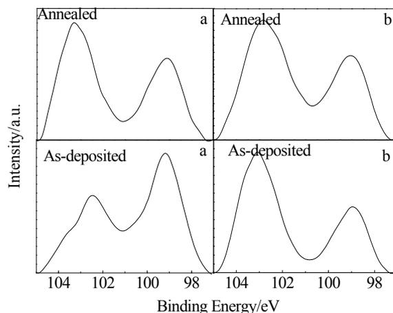
Fig.2 Si2p spectra for the as-deposited film and the annealed film,
