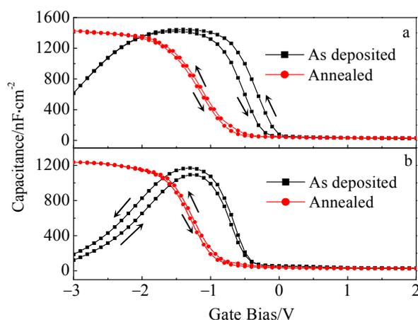
Fig.5 Capacitance characteristics of MIS capacitors made of the as-deposited film and the annealed film, respectively: (a) with a blocking layer, (b) without blocking layer
