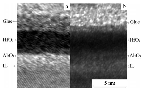
Fig.4 HRTEM images for the samples with blocking layer: (a) annealed and (b) as-deposited
