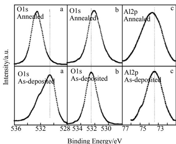
Fig.3 XPS spectra for the as-deposited film and the annealed film, respectively: (a) O1s spectra with a blocking layer, (b) O1s spectra without blocking layer, and (c) Al2p spectra
