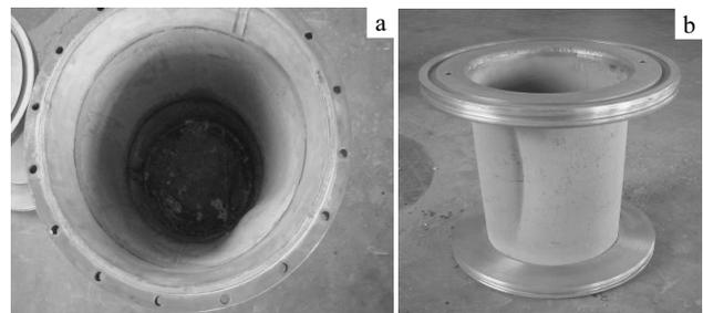
Fig.3 Photographs of broken porous cone (a) and tube (b)
