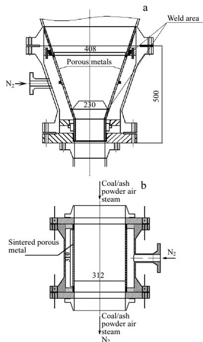
Fig.1 Porous cone (a) and tube (b)
