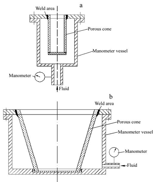
Fig.2 Schematic of breaking pressure test: (a) for tube; (b) for cone with overall dimension
