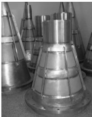
Fig.4 Photo of assembly with porous cone used in coal gasification
