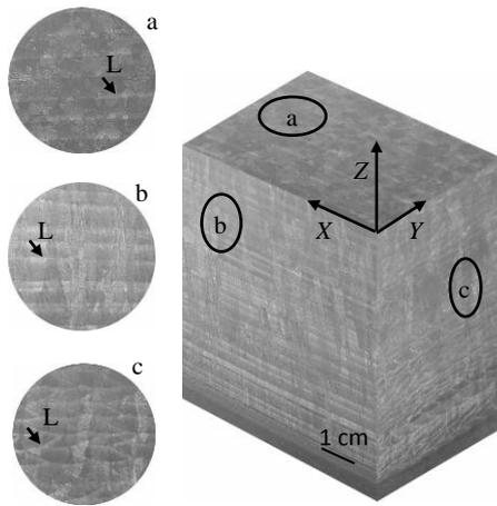
Fig.2 Macrograph of the Ti-6Al-4V bulk built by EBRM: (a) XY section, (b) XZ section, and (c) YZ section
