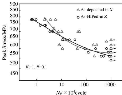
Fig.6 High cycle fatigue S-N curves of EBRM Ti-6Al-4V in X and Z directions
