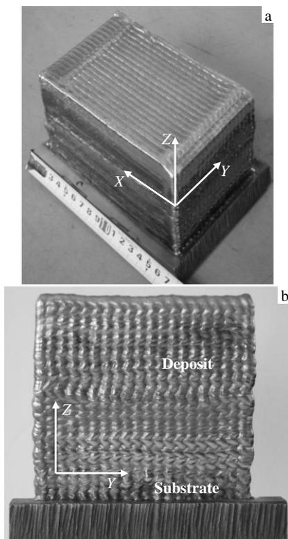
Fig.1 Ti-6Al-4V sample built by EBRM (150 mm × 100 mm × 100 mm)
