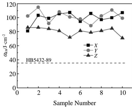
Fig.5 Room temperature Impact toughness  $\alpha_{ku}$  of Ti-6Al-4V as-HIPed in three directions (X, Y, Z); selected 10 samples on X, Y, Z directions, respectively (as Fig.2 show)
