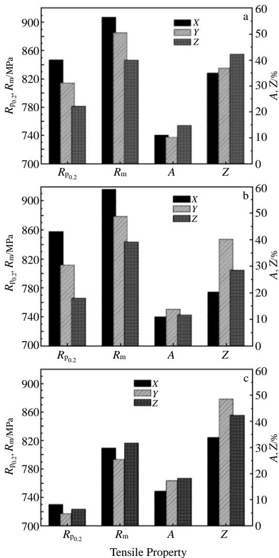
Fig.4 Tensile properties in three directions (X, Y, Z) of EBRM Ti-6Al-4V alloy under as-deposited (a), as-annealed (b), and as-HIPed (c) conditions
