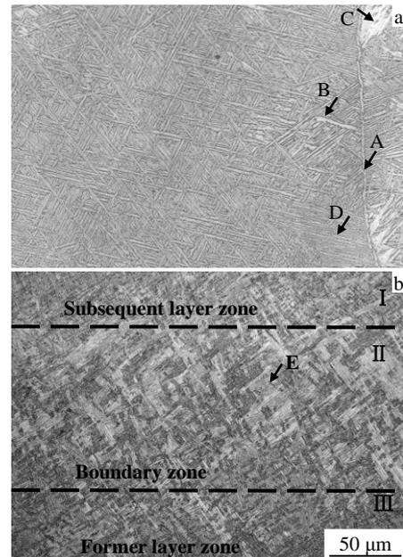
Fig.3 Microstructure of the EBRM Ti-6Al-4V: (a) weaved fine acicular  $\alpha$  laths,  $\alpha$  bunches and continuous grain boundary  $\alpha$ ; (b) microstructure around interlayer boundaries
