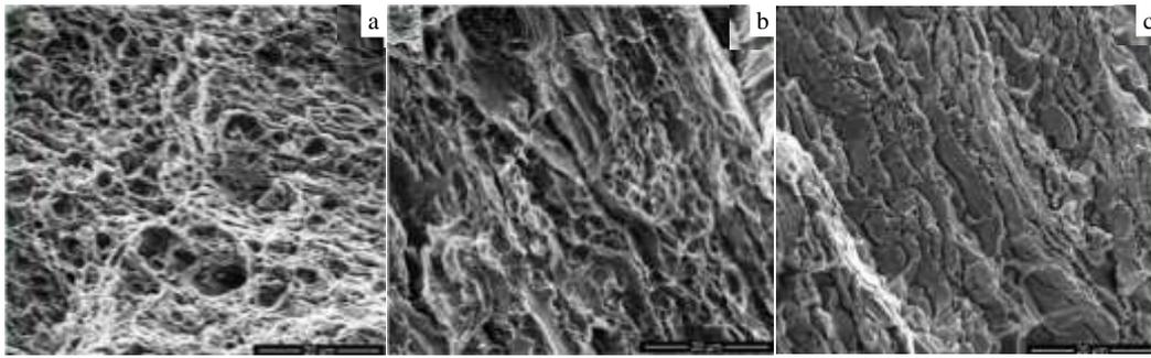
Fig.4 Fracture morphologies of extrusion bar (a), seamless pipe (b), and stripper plate (c)
