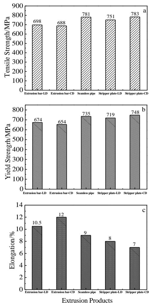
Fig.3 Mechanical properties in CD and LD of the different products: (a) tensile strength, (b) yield strength, and (c) elongation
