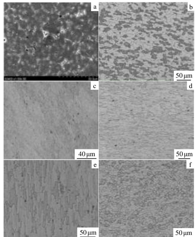
Fig.2 Microstructures of extrusion products: (a) billets as-deposited, (b) extrusion bar cross section, (c) extrusion bar longitudinal section, (d) seamless pipe longitudinal section, (e) stripper plate longitudinal section, and (f) stripper plate cross section
