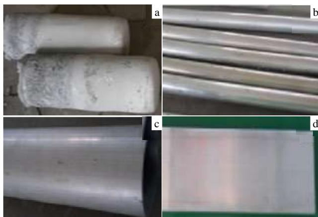
Fig.1 Billets and extrusion products: (a) billets as-deposited, (b) bar, (c) seamless pipe, and (d) stripper plate
