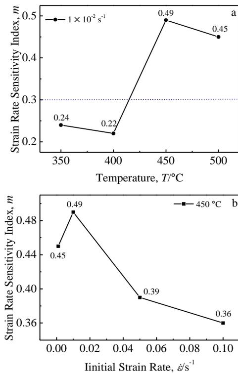
Fig.7 Line chart of the strain rate sensitivity index ( $m$ ) at different temperatures (a) and initial strain rates (b)
