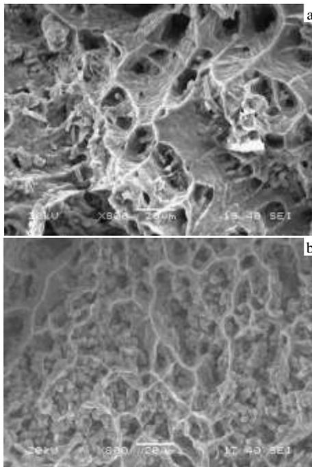
Fig.5 SEM images of high temperature tensile fracture with extension rate of 182% (a) and 330% (b)
