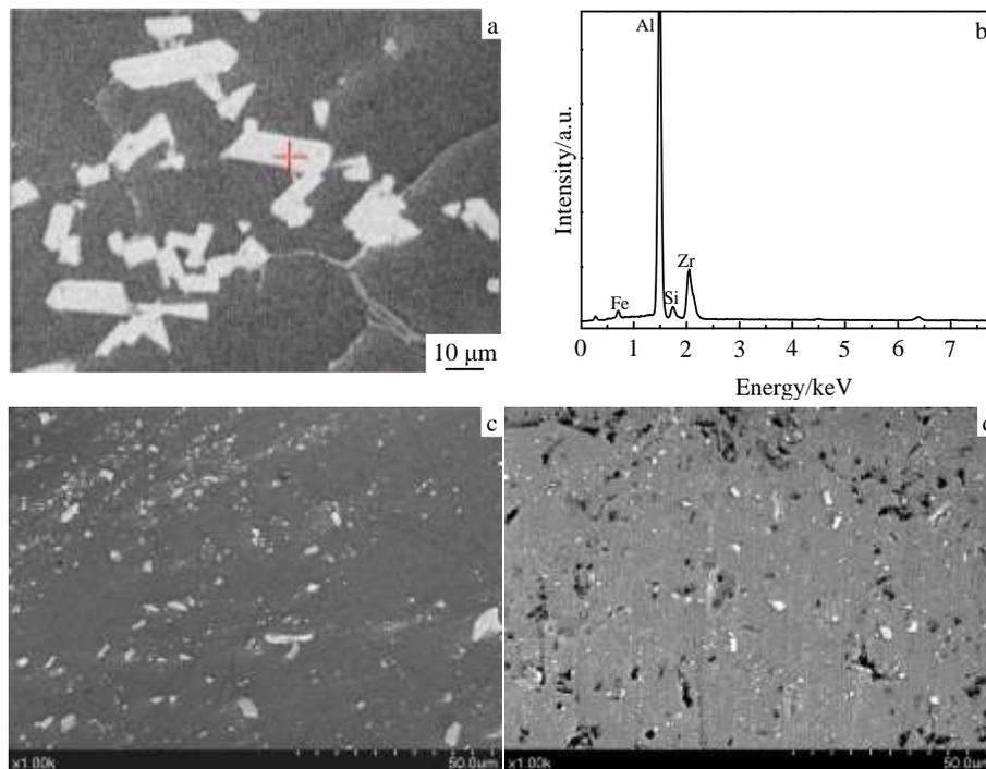
Fig.1 Microstructure of composites in different states and EDS spectrum under casting state: (a) casting states, (b) EDS of casting states, (c) forging states, and (d) FSP
