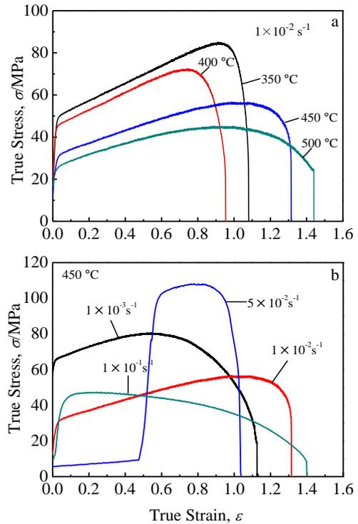
Fig.3 True stress-true strain curves of composite under different conditions: (a)  $\dot{\epsilon} = 1 \times 10^{-2} \text{ s}^{-1}$  and (b)  $T = 450 \text{ }^\circ\text{C}$
