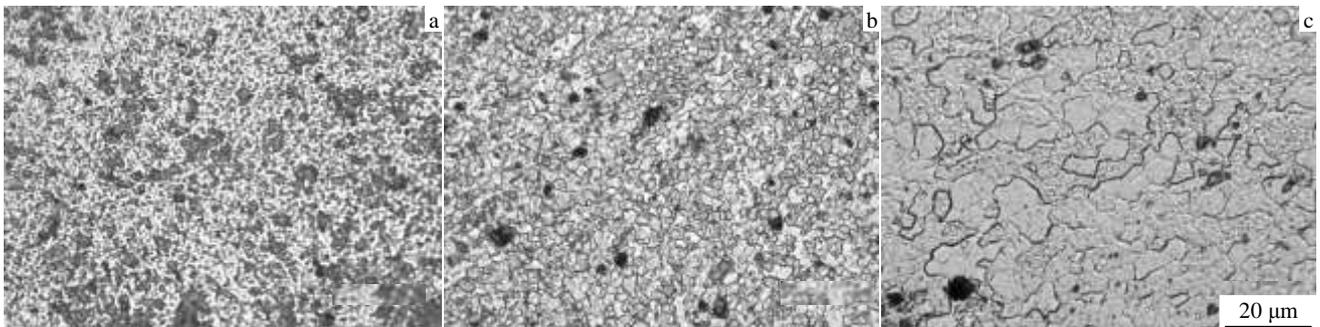
Fig.4 Microscopic images contrast of matrix grains with high temperature tension: (a) FSP before high temperature tensile experiment; (b) the drawing parts after high temperature tensile experiment; (c) the blessing part after high temperature tensile experiment
