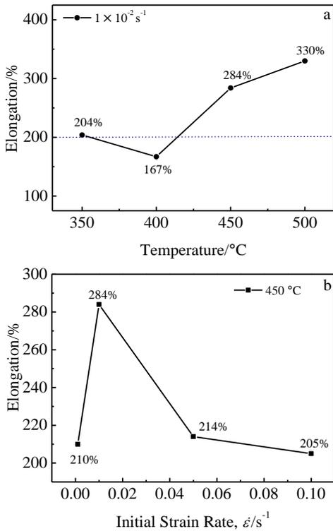
Fig.2 Effects of test temperature (a) and initial strain rate (b) on elongation of composites
