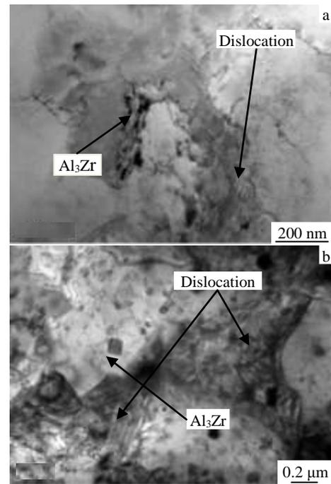
Fig.6 Dislocation of forged (a) and friction stirring state (b) of Al<sub>3</sub>Zr/6063Al composites
