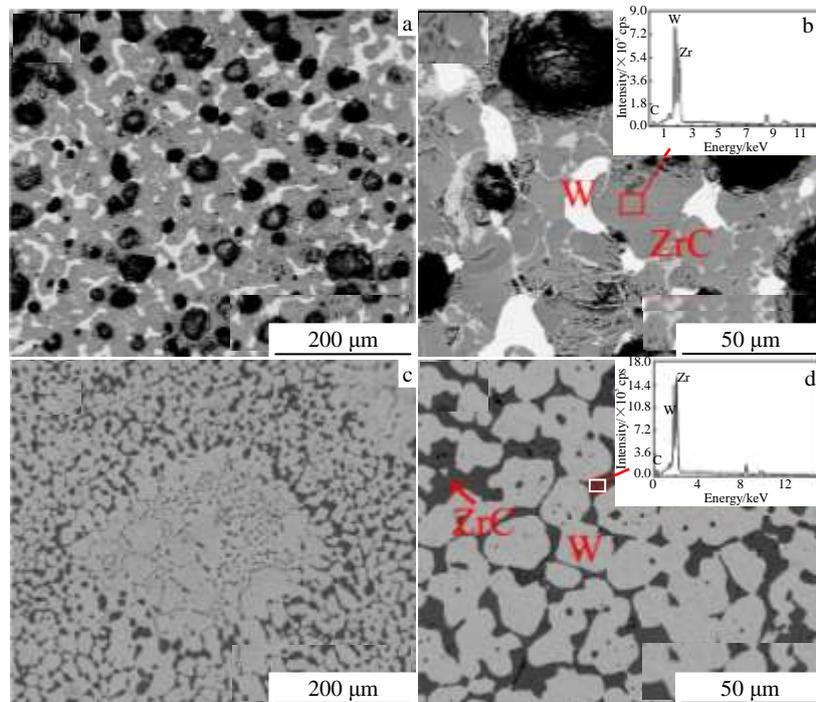
Fig.5 Backscattered electron images and EDS spectra of the two W/ZrC cermets after heat treatment at 2600 °C: (a, b) D-W/ZrC and (c, d) H-W/ZrC
