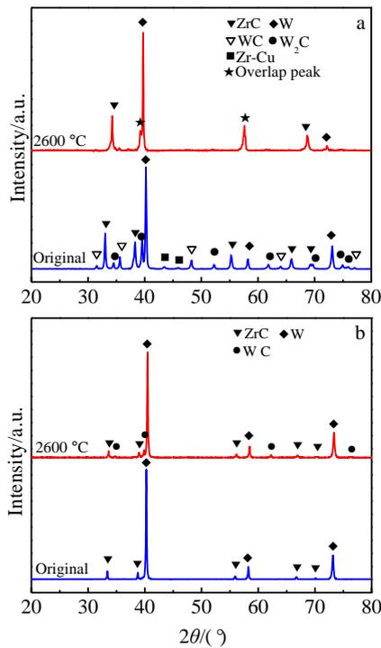
Fig.4 XRD patterns of D-W/ZrC (a) and H-W/ZrC (b) cermets obtained before and after heat treatment at 2600 °C
