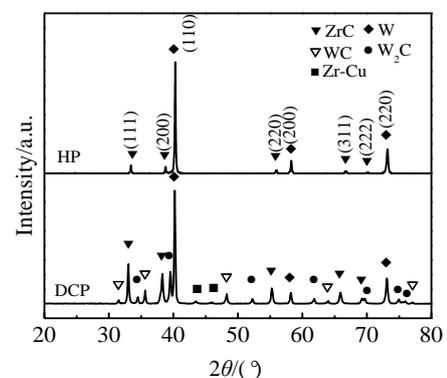
Fig.1 XRD patterns of W/ZrC cermets fabricated by different routes
