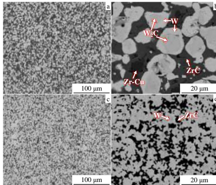
Fig.2 Backscattered electron images of W/ZrC cermets fabricated by different routes: (a, b) D-W/ZrC and (c, d) H-W/ZrC
