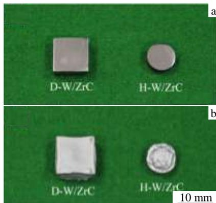
Fig.3 Optical images of W/ZrC cermets before (a) and after (b) heat treatment at 2600 °C
