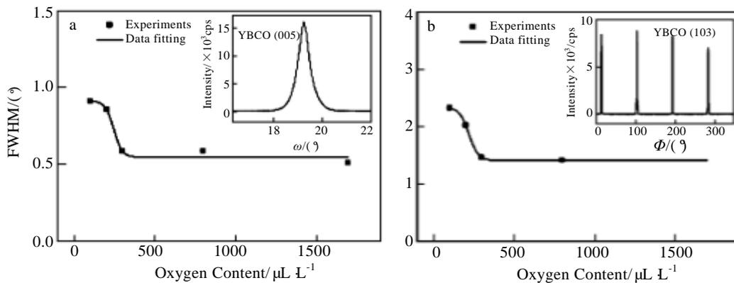
Fig.4 FWHM dependence of  $\omega$ - (a) and  $\Phi$  (b) scans on the oxygen content during heat treatment for YBCO films. (the insets are original results of  $\omega$ - and  $\Phi$  scans for the sample heat-treated at the oxygen content of 300  $\mu\text{L/L}$ )
