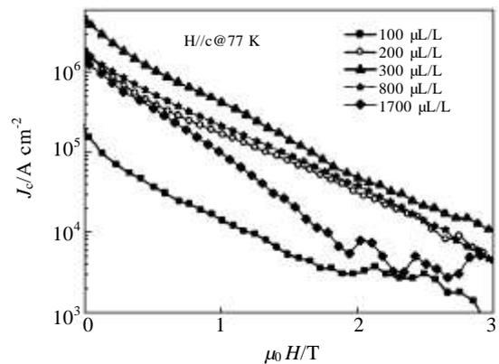
Fig.2  $J_c$ - $B$  relationship of YBCO films heat-treated under different oxygen contents
