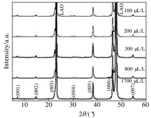
Fig.3  $\theta$ - $2\theta$  scan of XRD for YBCO films heat-treated under different oxygen contents
