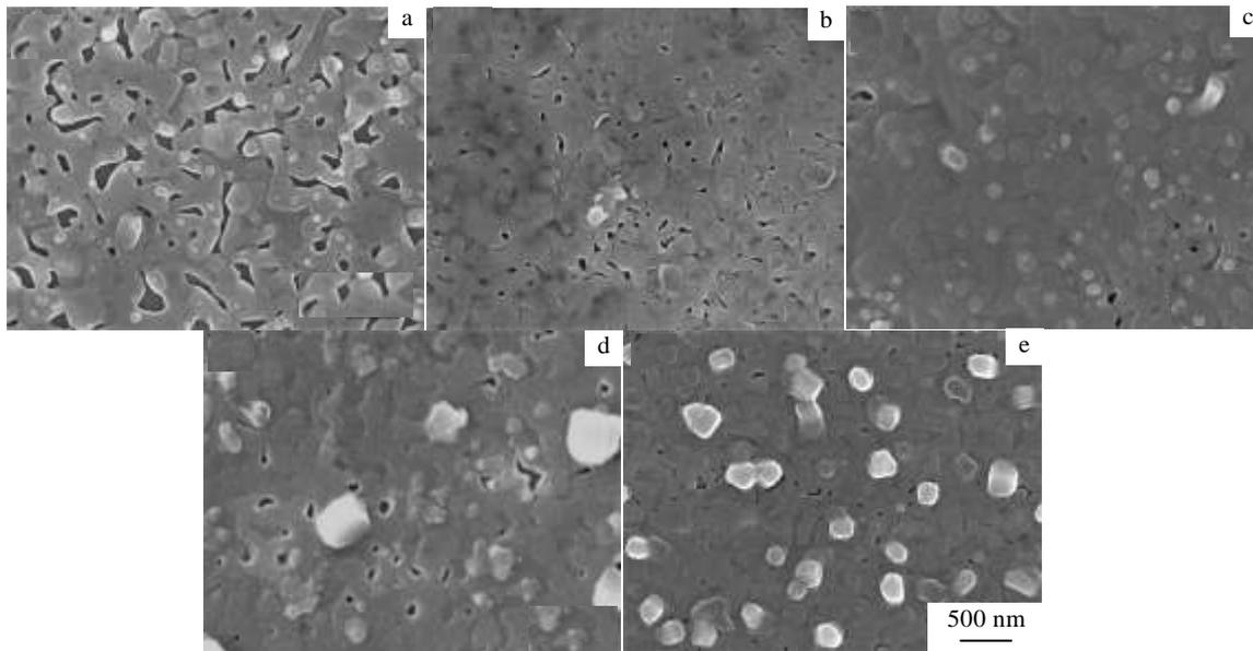
Fig.5 Surface morphologies of YBCO films heat-treated at the oxygen contents of 100  $\mu\text{L/L}$  (a), 200  $\mu\text{L/L}$  (b), 300  $\mu\text{L/L}$  (c), 800  $\mu\text{L/L}$  (d), and 1700  $\mu\text{L/L}$  (e)
