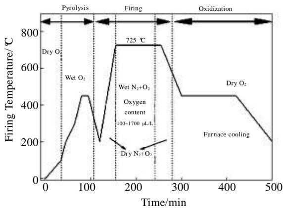
Fig.1 Profile of the heat treatment for preparing YBCO films
