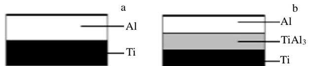
Fig.4 Schematic diagrams of diffusion of titanium and aluminum: (a) initial state and (b) annealing state
