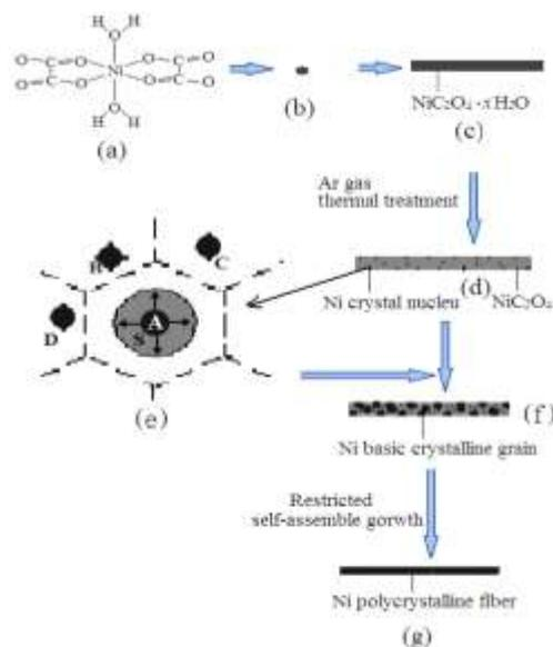
Fig.5 Schematic illustration of the formation process of nickel oxalate and nickel nano-fibers
