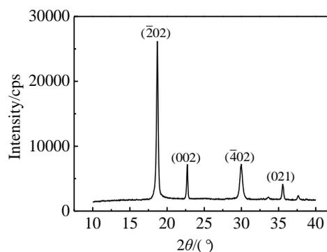
Fig.1 XRD pattern of nickel oxalate nano-fibers
