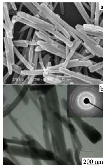
Fig.2 SEM (a) and TEM (b) images of nickel oxalate fibers
