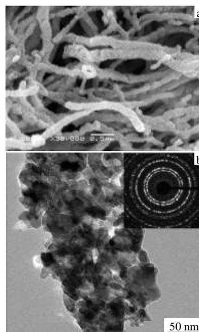
Fig.4 SEM (a) and TEM (b) images of nickel nano-fibers
