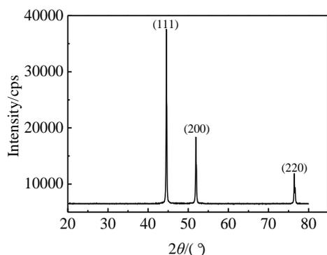
Fig.3 XRD pattern of nickel nano-fibers
