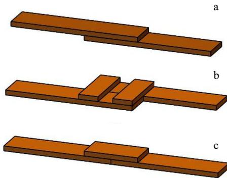
Fig.1 Schematic view of the electrical joint configuration for coated superconductor: (a) lapped joint, (b) bridged joint, and (c) butted joint
