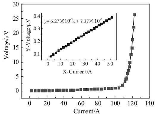
Fig.5  $V-I$  characteristic curve for the sample with length of 14 cm and thickness less than 10 μm
