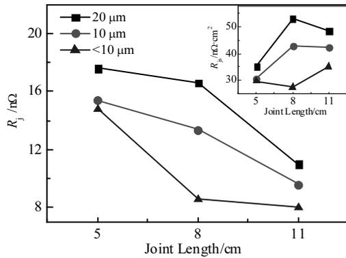
Fig.4 Chart of resistance and resistivity of joint samples for different joint length (solder thickness) (revealing that the resistance decreases with increasing the joint length or reducing the solder thickness. However, the joint sample with longer length has a larger resistivity)
