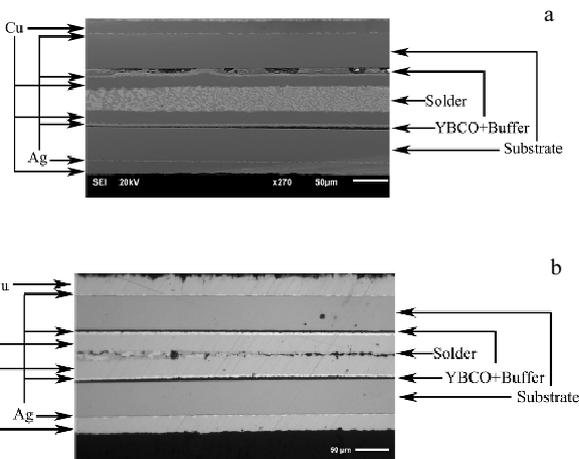
Fig.7 Micrographs of the transverse cross-section of jointed sample by SEM (a) and metallographic microscope (b)
