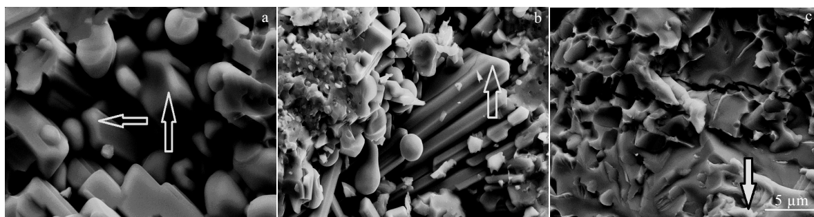
Fig.8 FESEM images nearby the interfacial region: (a) TiB 2 platelets pullout; (b) TiB platelets pullout; (c) ductile tearing of Ti
