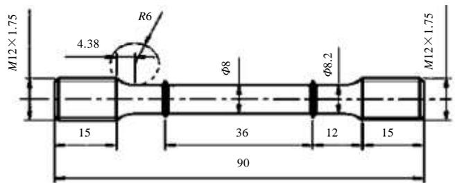
Fig.2 Geometry and size of sample (mm)
