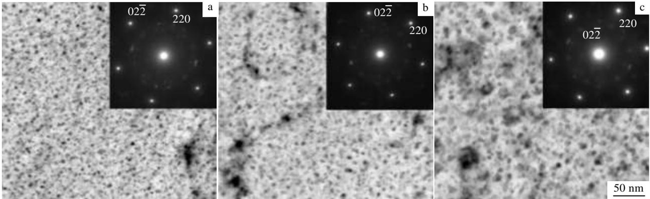
Fig.4 TEM micrographs and corresponding SAED patterns of the pre-retrogressed alloy under the external stress of 180 MPa and the stress-aging time of 4 h (a), 12 h (b), and 20 h (c)
