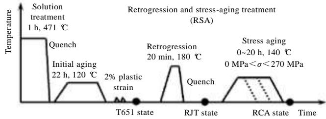
Fig.1 Retrogression and stress-aging treatment procedures
