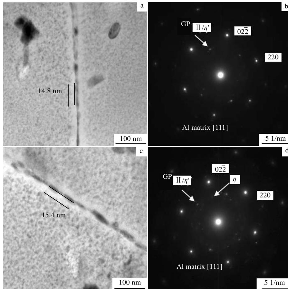
Fig.3 TEM micrographs (a, c) and corresponding SAED patterns (b, d) from  $\langle 111 \rangle$ Al projection of the studied alloy before and after retrogression heat treatment: (a, b) T651 state, as-received material; (c, d) RHT state, 20 min heat treatment at 180 °C
