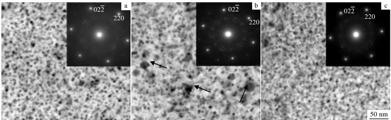
Fig.5 TEM micrographs and corresponding SAED patterns of the retrogressed alloy under the stress-aging time of 20 h and the external stresses of 90 MPa (a), 270 MPa (b), and 0 MPa (c)
