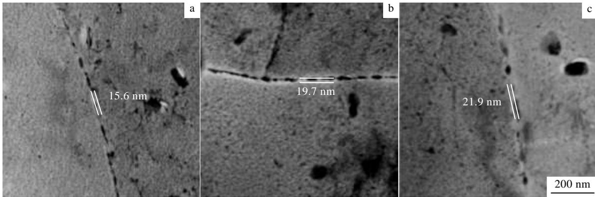
Fig.6 TEM micrographs of the retrogressed alloy under the external stress of 180 MPa and the stress-aging time of 4 h (a), 12 h (b), and 20 h (c)
