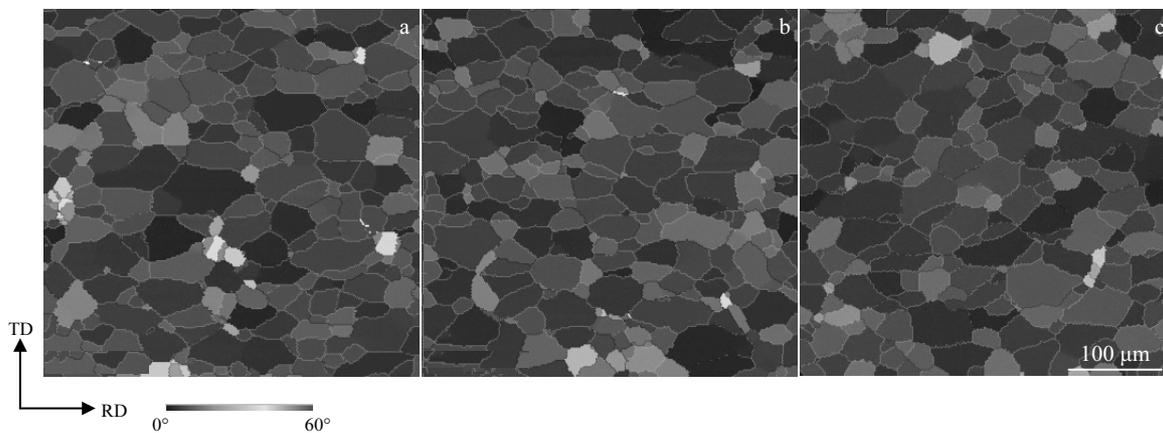
Fig.6 Crystal orientation maps of substrates annealed at 1200 °C/60 min: (a) sample #1, (b) sample #2, and (c) sample #3
