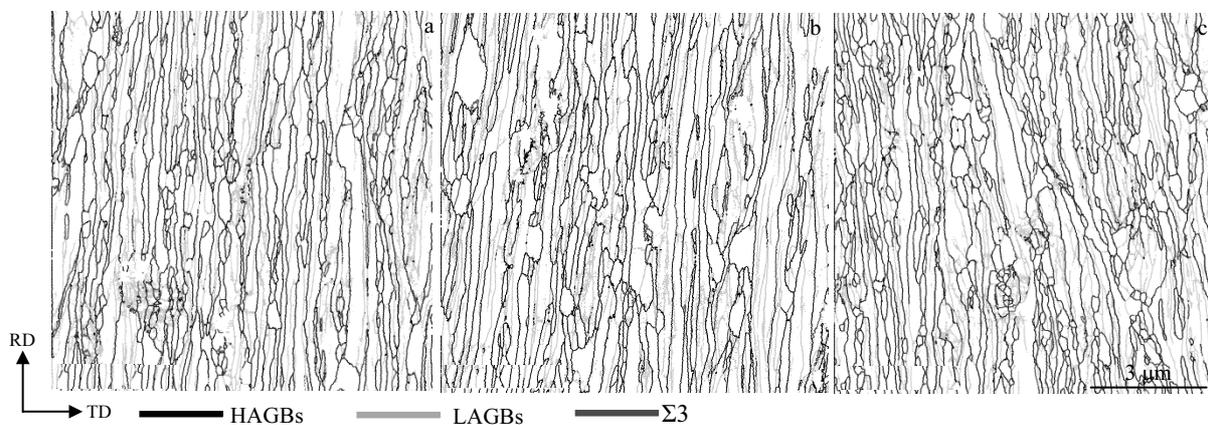
Fig.1 Grain boundary maps of the longitudinal section beneath the surface in Ni7W area: (a) sample #1, (b) sample #2, (c) sample #3 (measured by EBSD in a region of 10  $\mu$ m $\times$ 10  $\mu$ m with a step size of 0.02  $\mu$ m)
