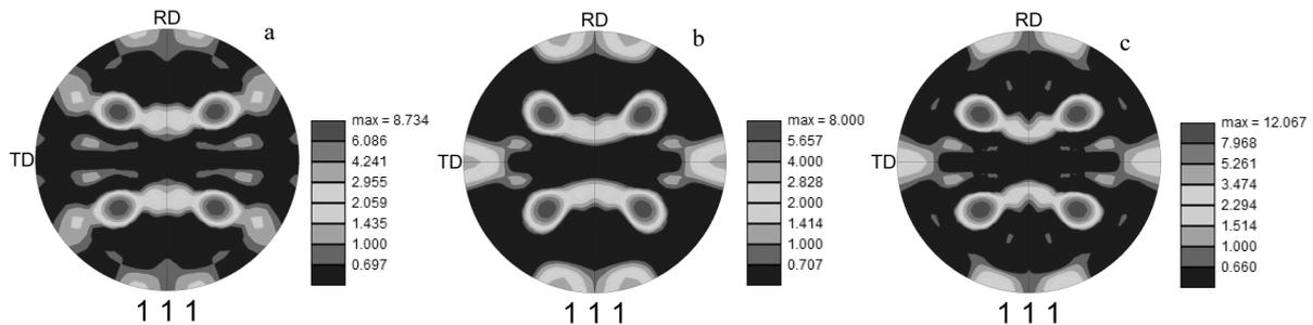
Fig.4 Pole figures of substrates annealed at 700 °C/30 min: (a) sample #1, (b) sample #2, and (c) sample #3 measured by EBSD on RD-TD section
