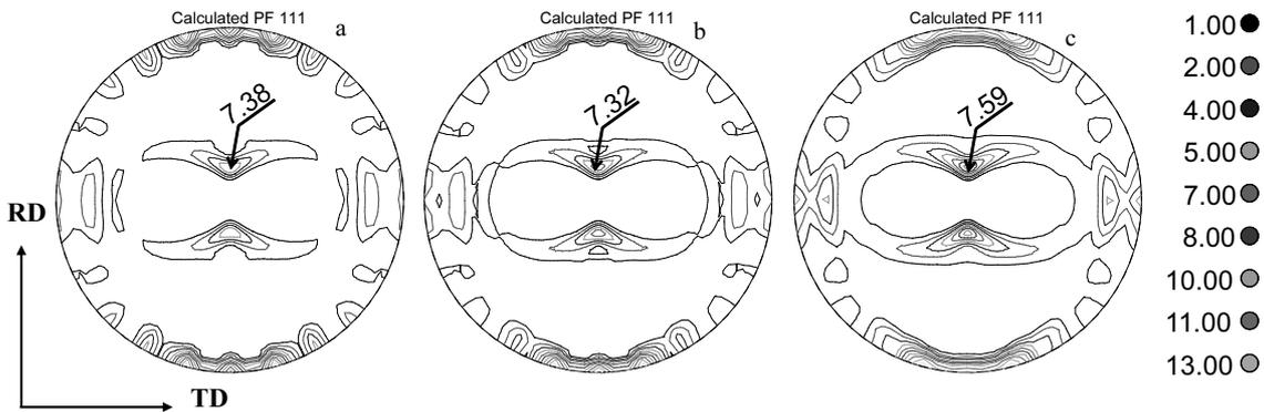
Fig.3 Pole figures of final-rolled substrates (80 μm): (a) sample #1, (b) sample #2, and (c) sample #3 measured by XRD on RD-TD section
