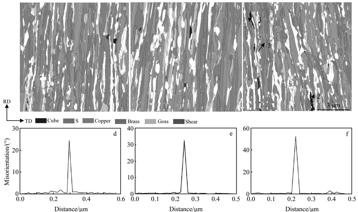
Fig. 2 Crystal orientation maps of the longitudinal section beneath the surface in Ni7W area (a~c): (a) sample #1, (b) sample #2, and (c) sample #3, measured by EBSD in a region of 10 μm×10 μm with a step size of 0.02 μm; the point to point misorientation between different grains (d~f): (d) Cube and S, (e) Cube and Copper, (f) Copper and S (along the black arrow marks numbered by 1, 2 and 3 in Fig. 2c)
