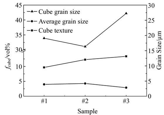
Fig.5 Grain sizes and cube texture of samples annealed at 700 °C/30 min
