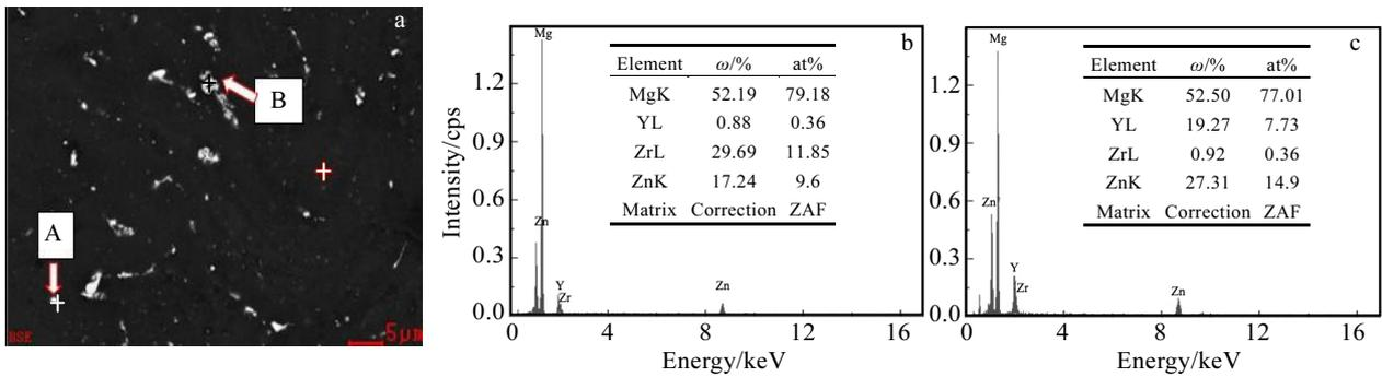
Fig.8 SEM image (a) and EDS results (b, c) of alloy aged at 200 °C/48 h: (b) point A in Fig.8a and (c) point B in Fig.8a
