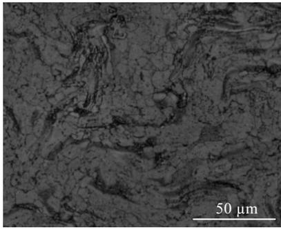
Fig.7 Microstructures of the alloy aged at 200 °C/48 h
