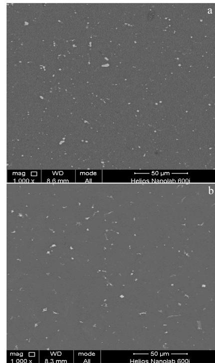
Fig.3 SEM images of the alloy solutionized at different parameters: (a) 500 °C/2 h and (b) 470 °C/5 h
