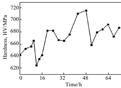
Fig.6 Hardness values of alloy with preservation time at 200 °C
