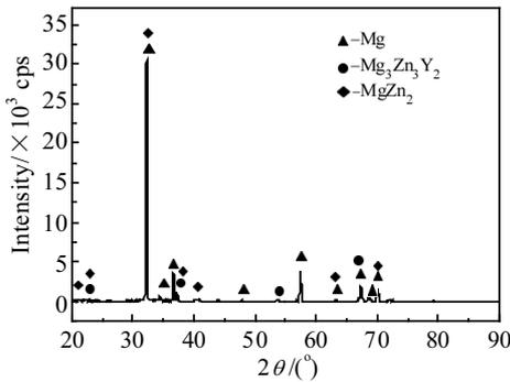
Fig.9 XRD pattern of alloy aged at 200 °C/48 h
