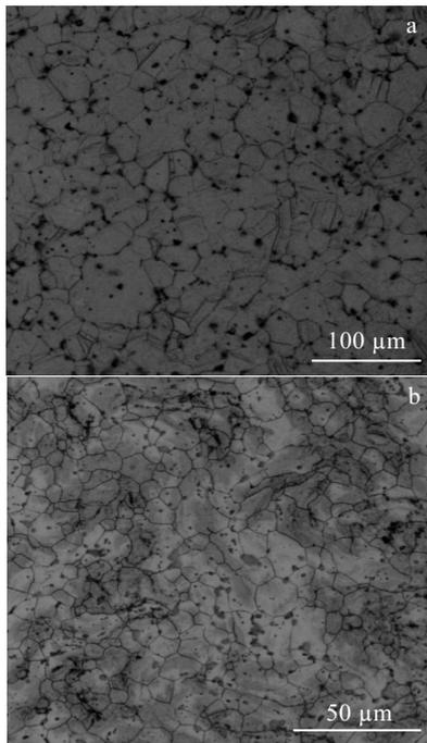
Fig.2 Microstructures of the alloy solutionized at different parameters: (a) 500 °C/2 h and (b) 470 °C/5 h
