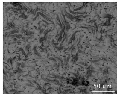
Fig.10 Microstructure of alloy after T6 treatment
