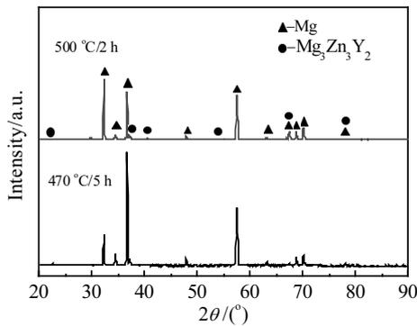
Fig.5 XRD patterns of alloy after solid solution treatment
