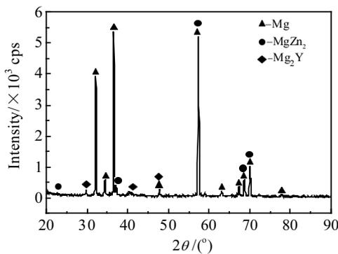
Fig.12 XRD pattern of alloy after T6 treatment
