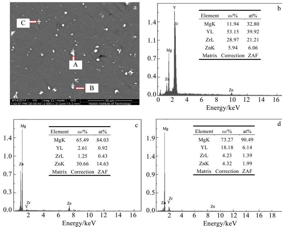
Fig.11 SEM image (a) and EDS results (b~d) of alloy after T6 treatment: (b) point A in Fig.11a; (c) point B in Fig.11a; (d) point c in Fig.11a
