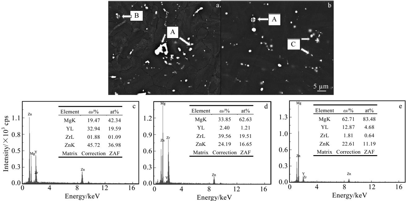
Fig.4 SEM images (a, b) and EDS results (c-e) of alloy after solid solution treatment: (a) 470 °C/5 h; (b) 500 °C/2 h; (c) point A in Fig.4b; (d) point B in Fig.4a; (e) point C in Fig.4b
