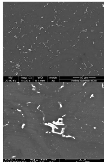
Fig.1 Microstructures of the as-extruded alloy
