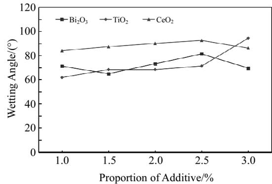
Fig.2 Wetting angle between Ag and SnO<sub>2</sub>
