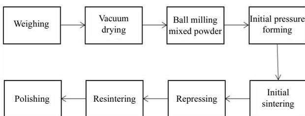
Fig.1 Manufacturing process of contact materials
