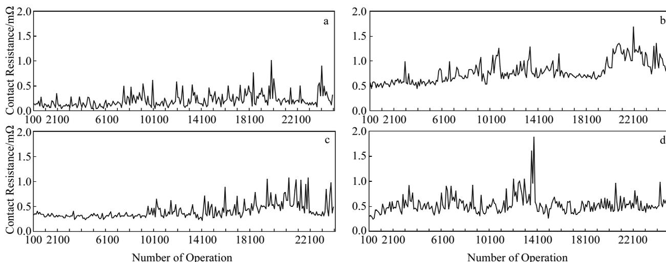
Fig.3 Contact resistance of Ag-SnO<sub>2</sub> contact materials doped with Bi<sub>2</sub>O<sub>3</sub> of different particle sizes: (a) 200 nm, (b) 500 nm, (c) 1 μm, and (d) 10 μm
