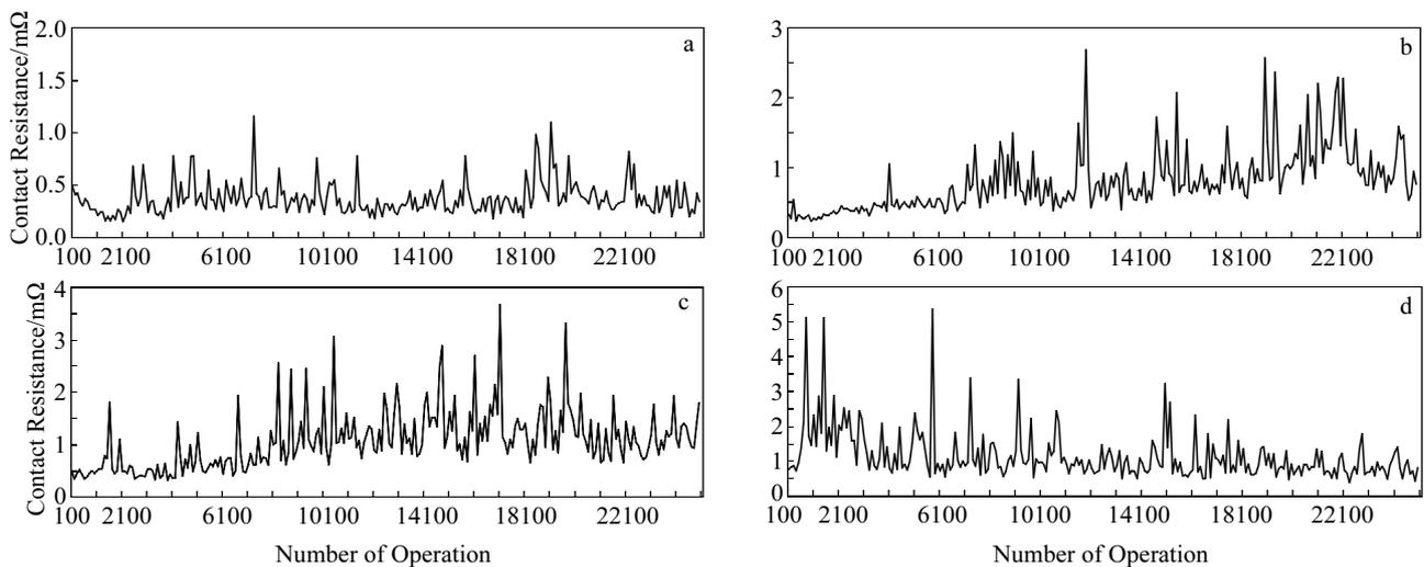
Fig.5 Contact resistance of Ag-SnO<sub>2</sub> contact materials doped with CeO<sub>2</sub> of different particle sizes: (a) 200 nm, (b) 500 nm, (c) 1 μm, and (d) 10 μm
