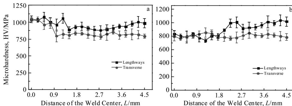
Fig.8 Microhardness distribution of 2325 welded joint (a) and 5B06 welded joint (b)
