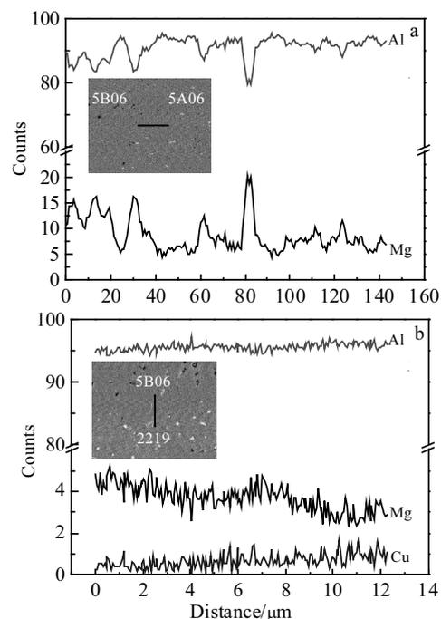
Fig.7 EDS line scanning results of the vicinity of 5B06 fusion zone: (a) 5B06-5A06 and (b) 5B06-2219
