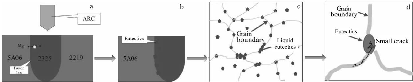
Fig.10 Schematic diagram of crack initiation: (a) the diffusion of alloy element, (b) eutectics production, (c) weld solidification, and (d) small cracks
