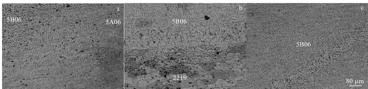
Fig.5 Typical microstructures of different zones in 5B06 weld: (a) microstructure on 5A06 side of fusion line, (b) microstructure on 2219 side of fusion line, and (c) the central of 5B06 weld
