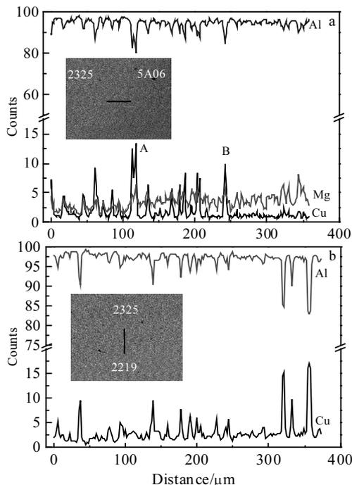
Fig.6 EDS line scanning results of the vicinity of 2325 fusion zone: (a) 2325-5A06 and (b) 2325-2219
