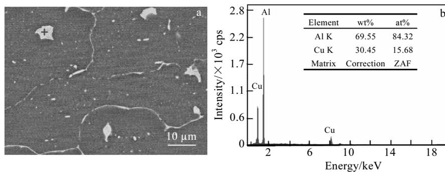
Fig.1 SEM image (a) and EDS spectrum (b) of 2219 base metals
