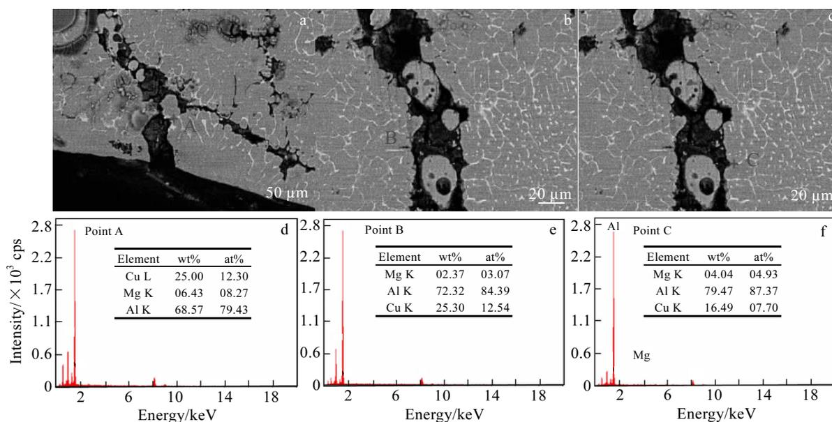
Fig.9 SEM images (a~c) and EDS analysis (d~f) of microstructure on the two side of crack
