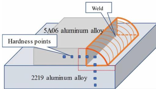
Fig.3 Schematic diagram of metallographic preparation and hardness tests
