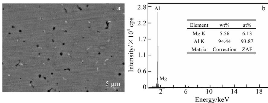
Fig.2 SEM image (a) and EDS spectrum (b) of 5A06 base metals
