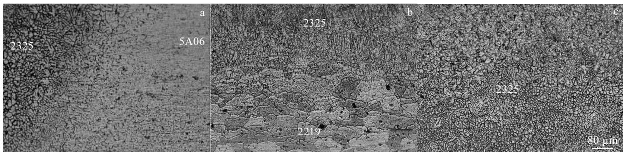
Fig.4 Typical microstructures in different zones of 2325 weld: (a) 5A06 side of fusion line, (b) 2219 side of fusion line, and (c) the center of 2325 weld
