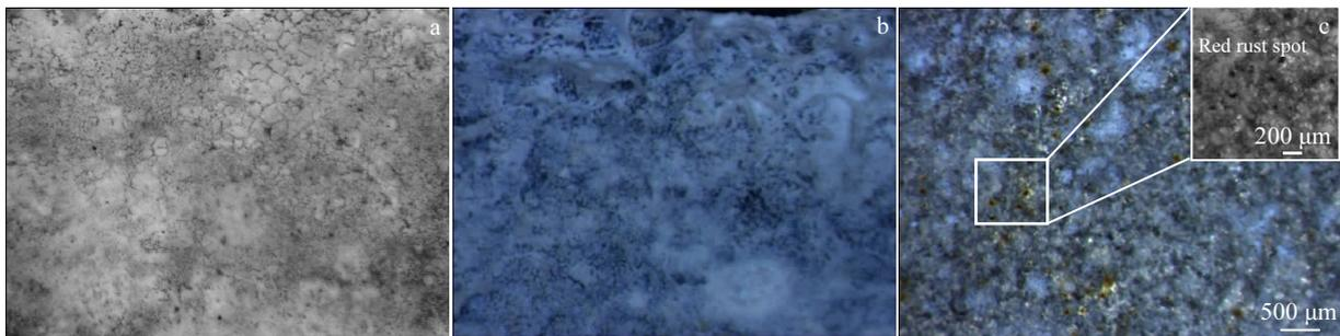
Fig.5 Macroscopic corrosion morphologies of the Zn55Al coating (a), Zn15Al coating (b), and Al coating (c) after 20 d immersion test in the 3.5 wt% NaCl solution at room temperature
