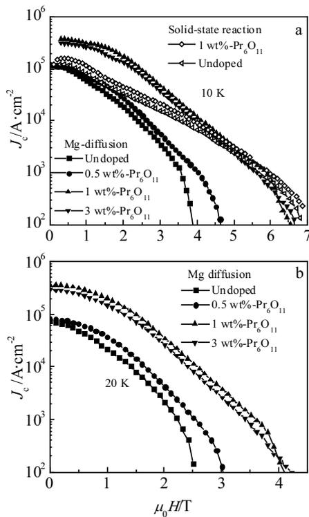
Fig.3 Magnetic field dependence of the critical density  $J_c$  properties at 10 K (a) and at 20 K (b)
