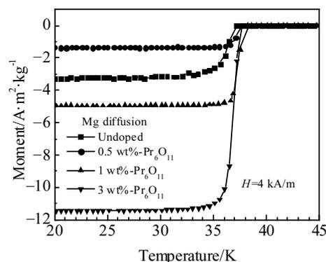
Fig.2 Temperature dependence of the magnetization measured at 4 kA/m
