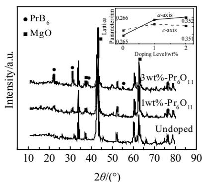
Fig.1 XRD patterns of the  $\text{Pr}_6\text{O}_{11}$ -doped  $\text{MgB}_2$  samples after heating at 850 °C for 24 h (Inset:  $a$ ,  $c$ -axis lattice parameters of  $\text{MgB}_2$ )
