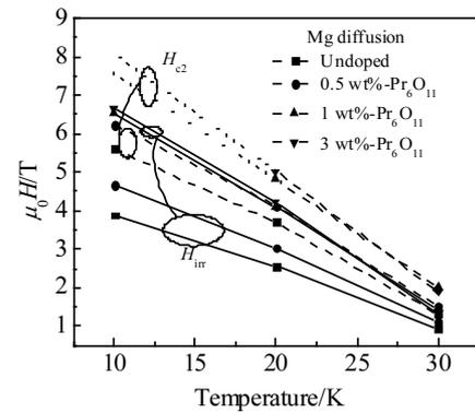
Fig.4 Temperature dependence of the irreversibility field  $H_{irr}$  and upper critical field  $H_{c2}$
