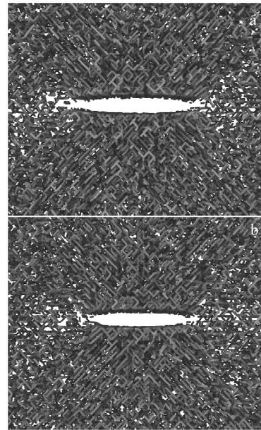
Fig.4 Atomic bond of crack tip of TiAl specimen with different Al contents: (a) 42 at% and (b) 48 at% (red represents Ti atomic bond, and blue represents Al atomic bond)
