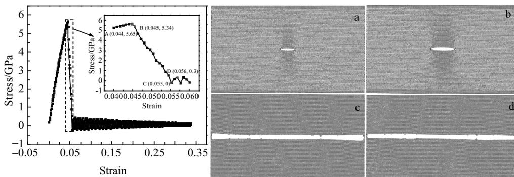
Fig.3 Stress-strain curves of TiAl specimen with Al content of 48 at% (atomic color from green to red represent stress value increasing): Fig.3a~3d corresponding to point A~D of the inset of stress-strain curve
