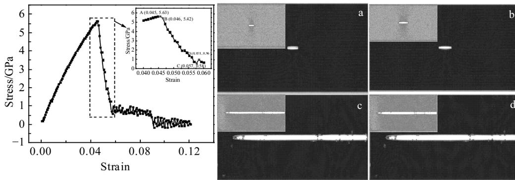
Fig.2 Stress-strain curves of TiAl specimen with Al content of 42 at% (atomic color from green to red represent stress value increasing): Fig.2a~2d corresponding to point A~D of the inset of stress-strain curve
