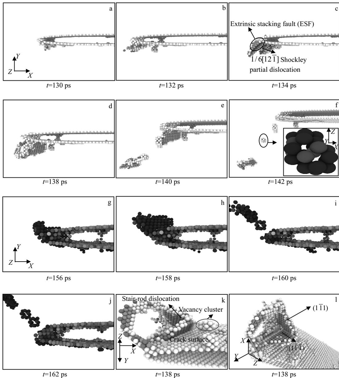
Fig.6 Defect evolution at crack tips with Al content of 42 at%
