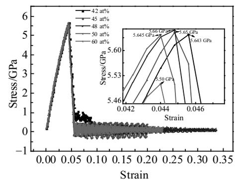
Fig.5 Stress-strain curves of TiAl specimen with different Al contents
