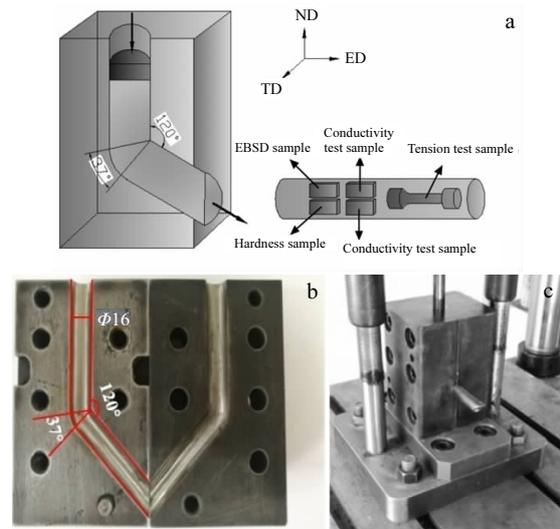
Fig.1 Principle of equal-channel angular pressing (a), die structure (b), and actual assembly drawing (c)
