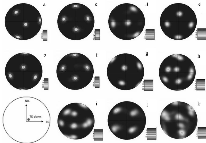
Fig.5  $\{111\}$  pole figures of samples after ECAP for several passes by route A, Bc and C: (a) initial condition; (b) 1 pass; (c) 2 passes of route A; (d) 2 passes of route Bc; (e) 2 passes of route C; (f) 4 passes of route A; (g) 4 passes of route Bc; (h) 4 passes of route C; (i) 6 passes of route A; (j) 6 passes of route Bc; (k) 6 passes of route C
