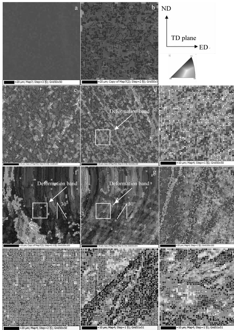
Fig.2 Orientation image microscopy (OIM) images of single crystal copper samples after ECAP for several passes through different routes: (a) 0 pass, (b) 1 pass, (c) 2 passes of route A, (d) 4 passes of route A, (e) 6 passes of route A, (f) 2 passes of route Bc, (g) 4 passes of route Bc, (h) 6 passes of route Bc, (i) 2 passes of route C, (j) 4 passes of route C, and (k) 6 passes of route C
