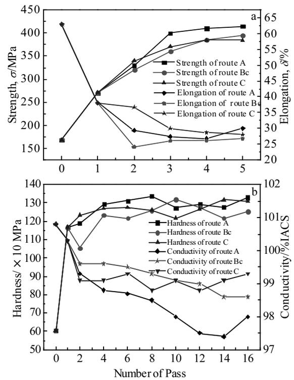
Fig.3 Mechanical properties of different ECAP passes by route A, Bc and C (a); relationship between ECAP pass, hardness and conductivity (b)
