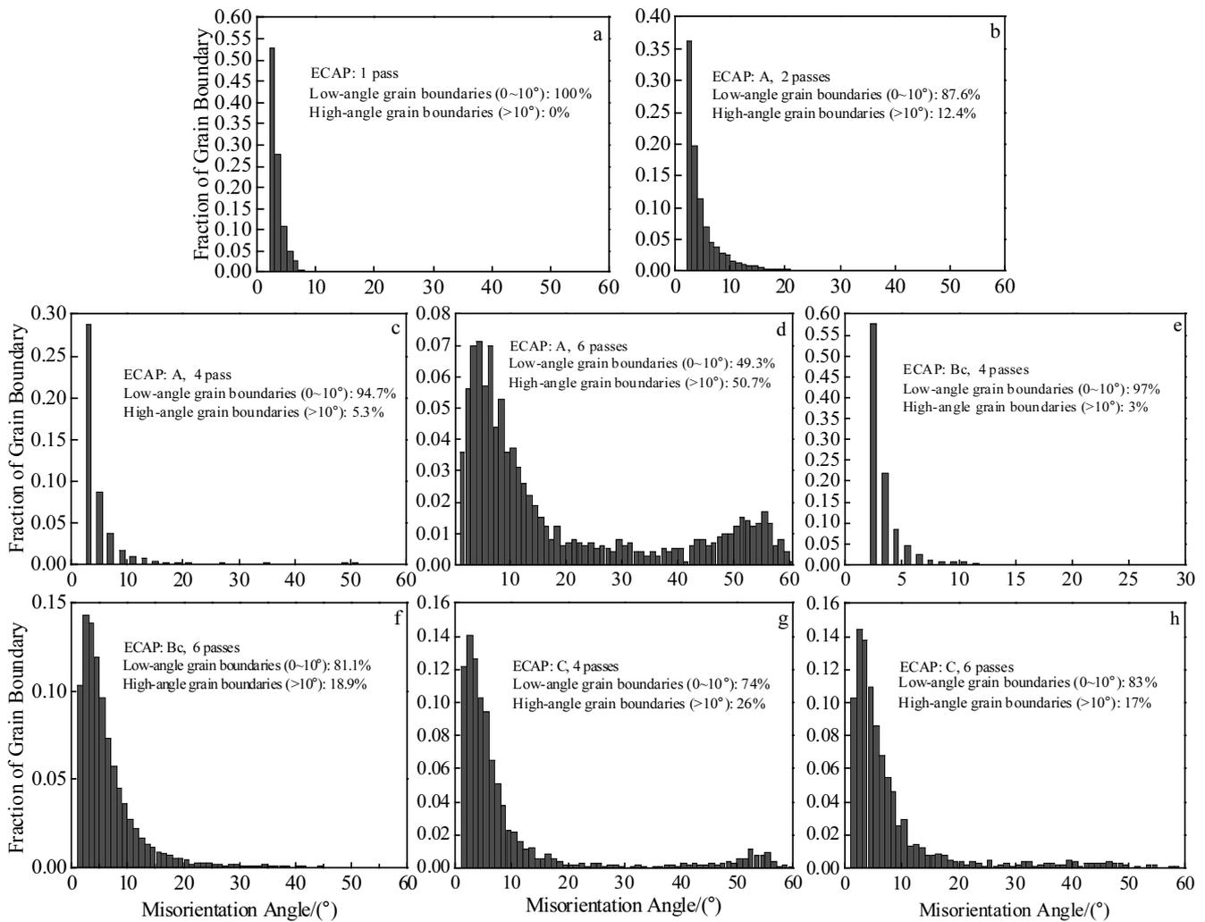
Fig.4 Misorientation angle distribution of Cu samples after several ECAP passes by route A, Bc and C: (a) 1 pass; (b) 2 passes of route A; (c) 4 passes of route A; (d) 6 passes of route A; (e) 4 passes of route Bc; (f) 6 passes of route Bc; (g) 4 passes of route C; (h) 6 passes of route C
