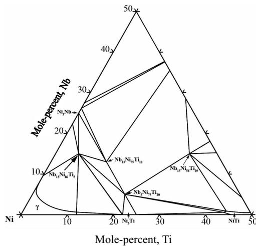
Fig.1 Calculated isothermal section at 1273 K in the Ni-Nb-Ti system using the thermodynamic parameters of Matsumoto et al<sup>[20]</sup>
