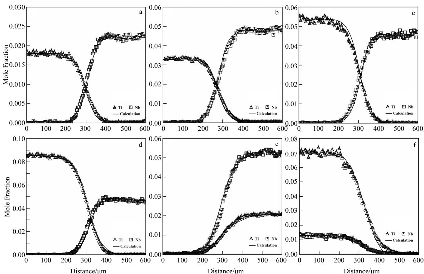
Fig.3 Comparison between the calculated and the measured concentration profiles for the six diffusion couples annealed at 1273 K for 432 000 s: (a) A1, (b) A2, (c) A3, (d) A4, (e) B1, and (f) B2
