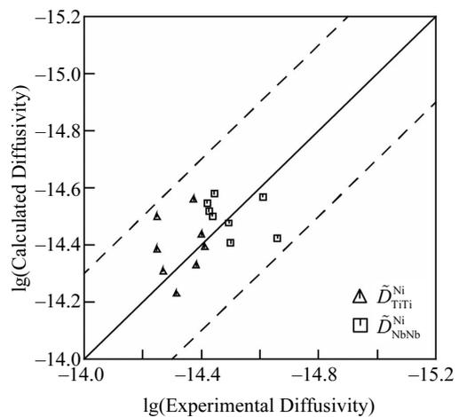
Fig.2 Comparison between the calculated major interdiffusion coefficients of the fcc Ni-Nb-Ti system at 1273 K and the experimental values (dashed lines refer to the diffusion coefficients with a factor of 2 or 0.5 from the model-predicted ones)
