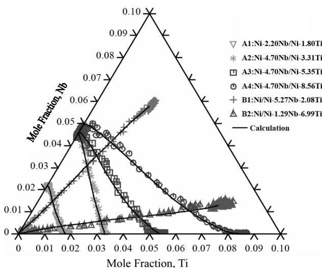
Fig.4 Calculated diffusion paths for various ternary Ni-Nb-Ti diffusion couples annealed at 1273 K for 432 000 s, compared with the experimental data measured in this work
