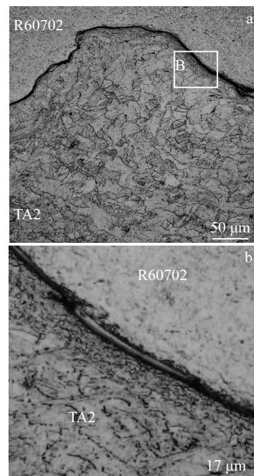
Fig.5 Microstructures of TA2 near the interface (a) and enlarged view of fine equiaxed grain zone of position B in Fig.5a (b)
