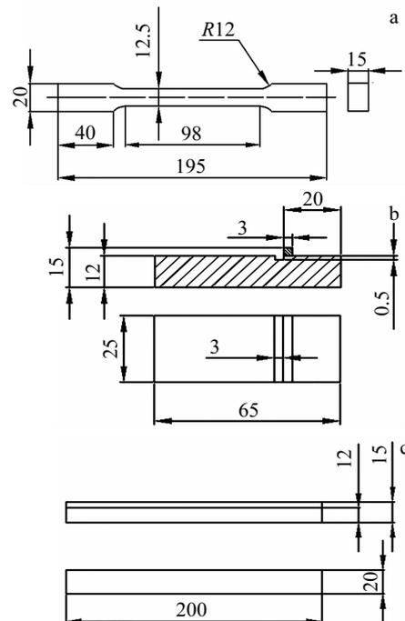
Fig.2 Dimensions of tensile test specimen (a), shear test specimen (b), and bending test specimen (c) (mm)
