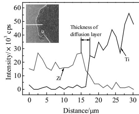
Fig.4 Element line scan results of bonding interface
