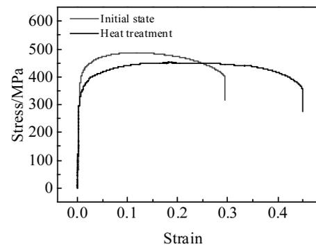
Fig.11 Stress-strain curves of the explosively welded R60702/TA2 composite plate before and after heat treatment
