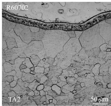
Fig.9 OM microstructure of TA2 near the interface after heat treatment
