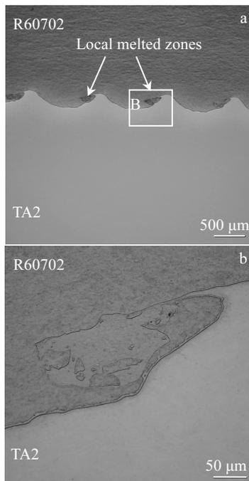
Fig.3 OM microstructures of bonding interface of R60702/TA2 composite plate (a) and enlarged view of position B in Fig.3a (b)
