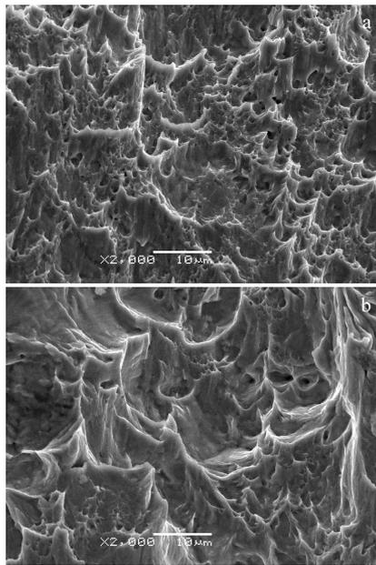
Fig.14 Fractographs of shear test specimen before (a) and after (b) heat treatment
