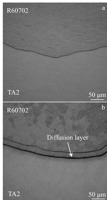
Fig.7 OM images of bonding interface before (a) and after (b) heat treatment
