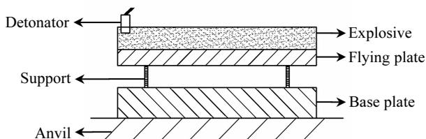
Fig.1 Parallel layer arrangement of explosive welding process
