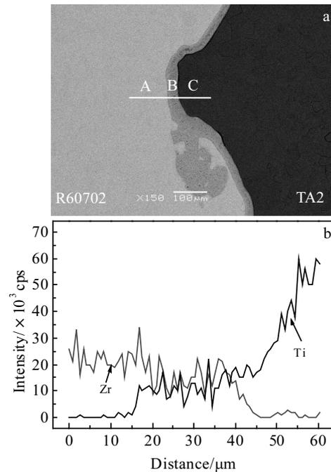
Fig.8 EDS analysis path (a) and line scan results across the bonding interface (b) after heat treatment
