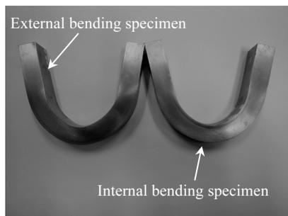
Fig.15 Specimens after bending test
