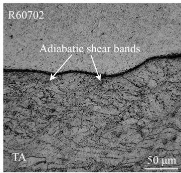
Fig.6 Adiabatic shear bands in TA2 side
