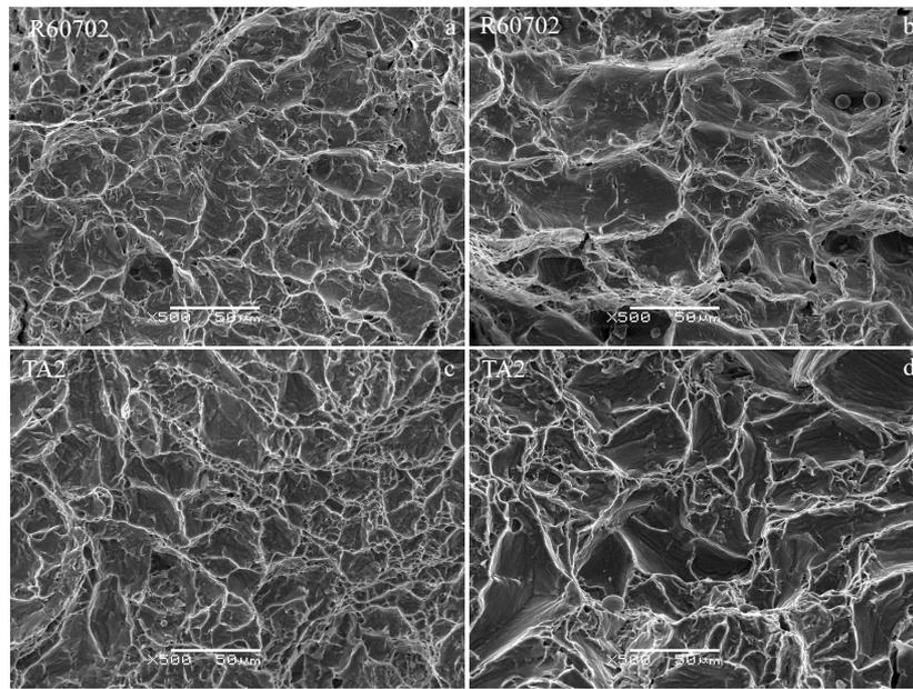
Fig.12 Tensile fractographs of R60702 before (a) and after (b) heat treatment; TA2 before (c) and after (d) heat treatment
