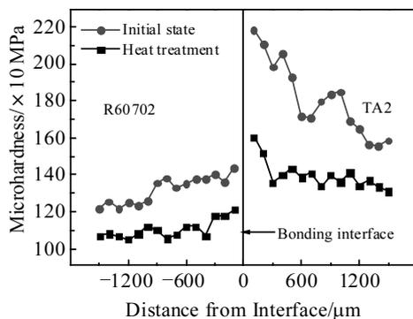
Fig.10 Microhardness profile near the bonding interface before and after heat treatment
