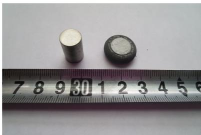
Fig.1 Typical photos of the specimens before and after isothermal compression tests
