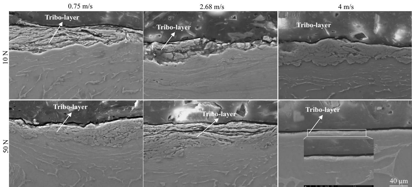
Fig.5 Cross-section morphologies of worn surfaces of the aluminized Ti-6Al-4V under 10 and 50 N at different sliding velocities
