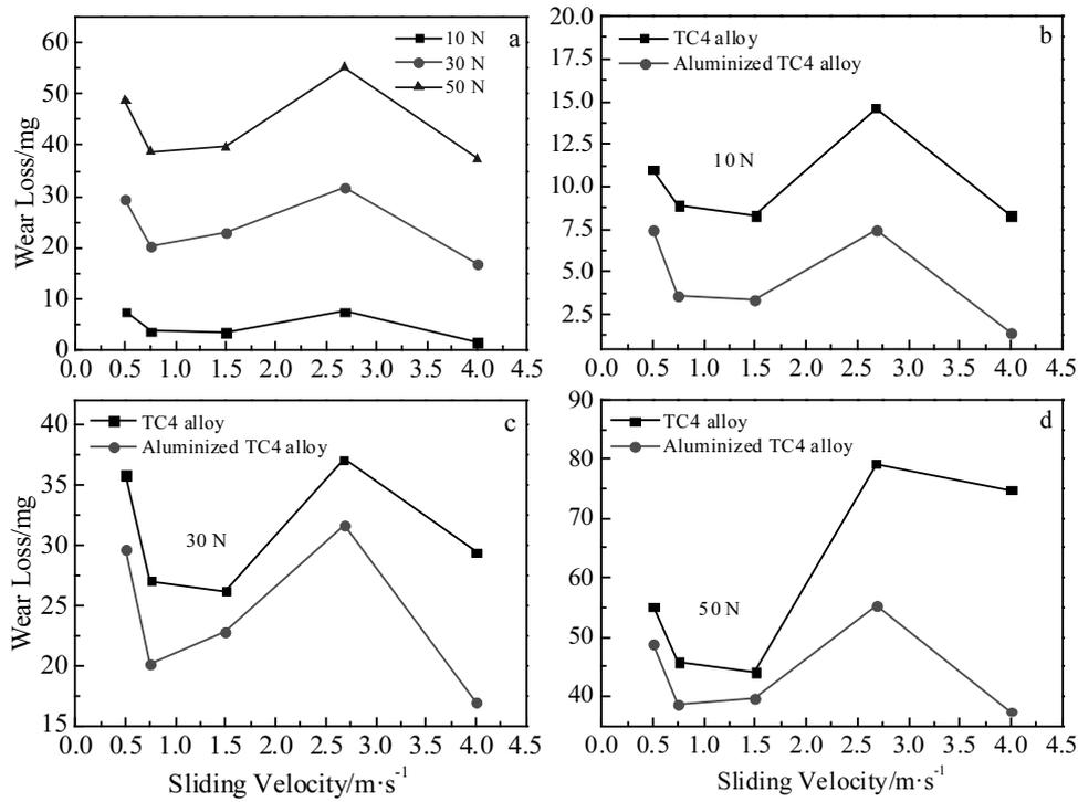
Fig.2 Wear losses of aluminized Ti-6Al-4V alloy (a) and wear loss comparison (b~d) between the aluminized and uncoated Ti-6Al-4V alloys
