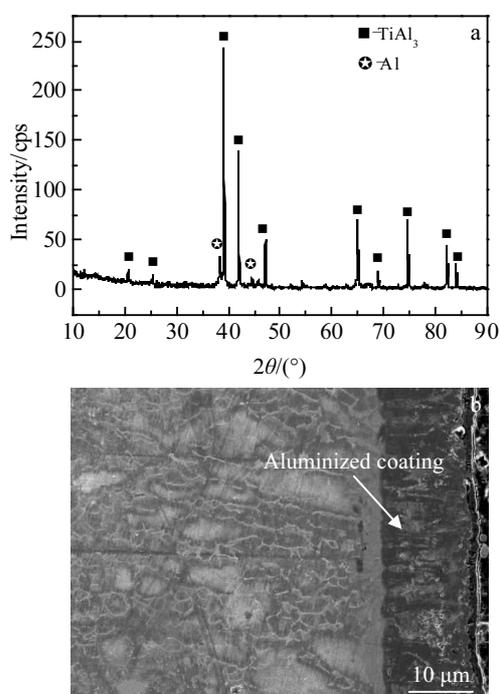
Fig.1 XRD pattern (a) and cross-section morphology (b) of the aluminized coating on Ti-6Al-4V alloy
