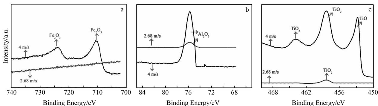
Fig.6 XPS spectra of Fe 2p (a) , Al 2p (b) and Ti 2p (c) on the worn surface of the aluminized coating at a normal load of 50 N and sliding speeds of 2.68 and 4 m/s
