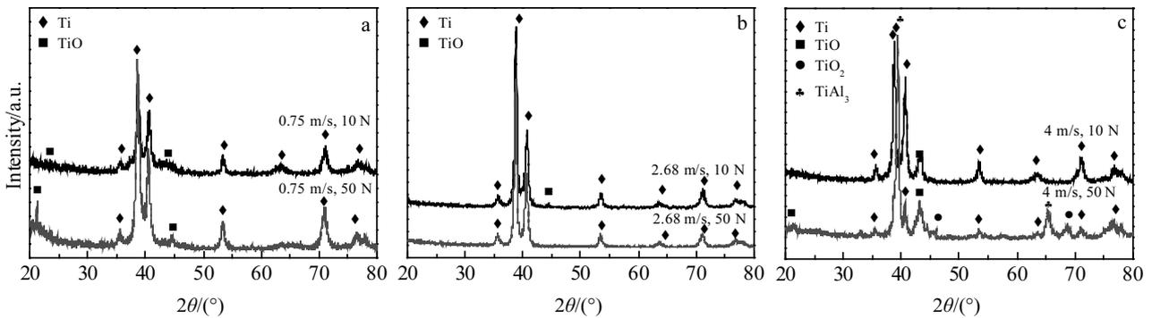
Fig.3 XRD patterns of worn surfaces of aluminized Ti-6Al-4V alloy sliding under various conditions: (a) 0.75 m/s, (b) 2.68 m/s, and (c) 4 m/s
