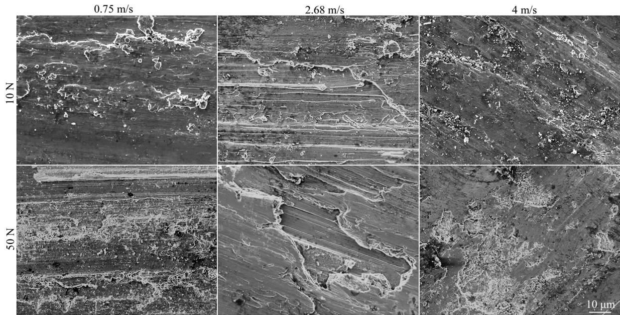
Fig.4 Morphologies of worn surfaces of the aluminized Ti-6Al-4V under 10 and 50 N at different sliding velocities
