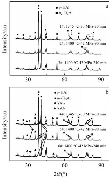
Fig.3 XRD patterns of Ti45Al (a) and Ti45Al0.3Y (b) under different VHPS parameters
