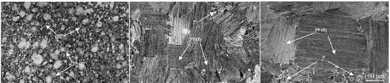
Fig.4 OM images of Ti45Al alloy processed under different VHPS parameters: (a) 1# 1345 °C-30 MPa-30 min; (b) 2# 1400 °C-42 MPa-90 min; (c) 3# 1400 °C-42 MPa-240 min
