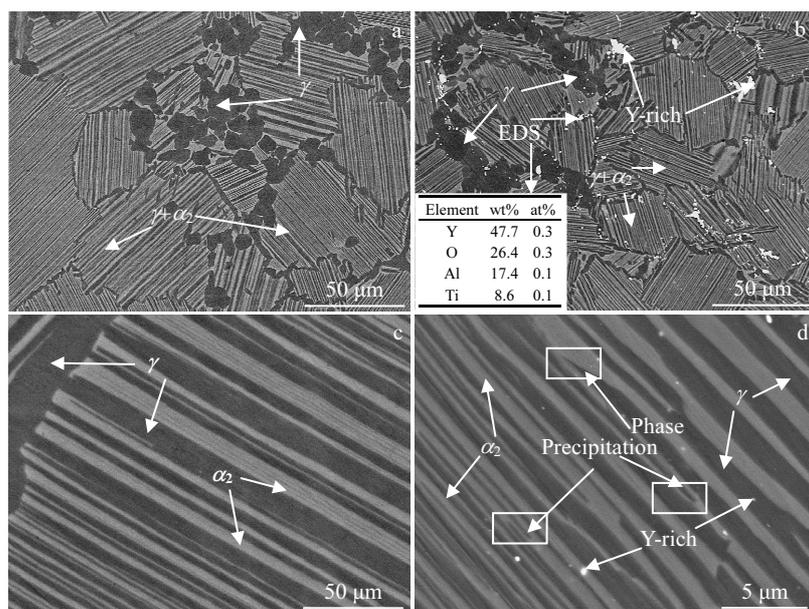
Fig.6 BSE images of the TiAl-based alloy processed at 1400 °C for 90 min: (a, c) sample 2# and (b, d) sample 5#
