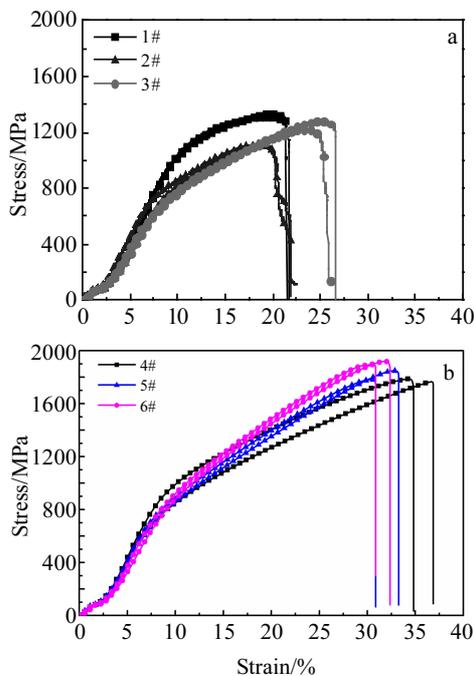
Fig.7 Compression curves of Ti45Al (a) and Ti45Al0.3Y(b) alloys processed under different VHPS conditions
