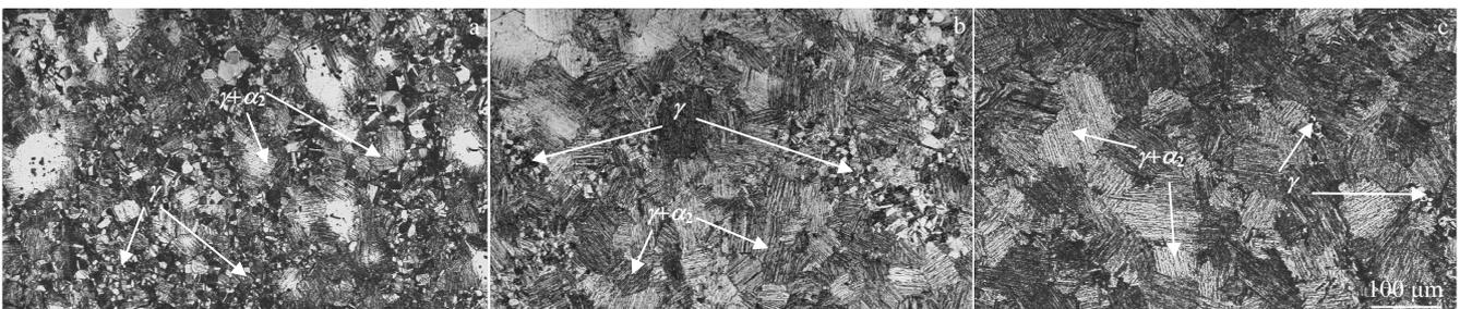
Fig.5 OM images of Ti45Al0.3Y alloy processed under different VHPS process parameters: (a) 4# 1345 °C-30 MPa-30 min; (b) 5# 1400 °C-42 MPa-90 min; (c) 6# 1400 °C-42 MPa-240 min
