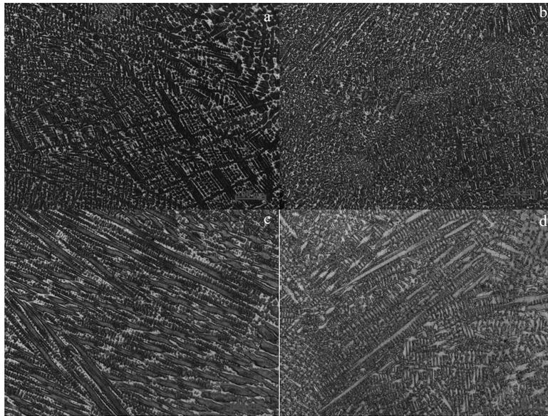
Fig.8 Microstructures of the as-welded joint: (a) area A, (b) area B, (c) area C, and (d) area D
