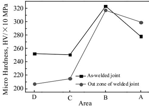
Fig.7 Micro-hardness distributions of the spun serrated groove
