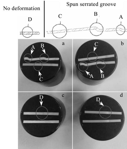
Fig.6 Inlaid specimens of serrated grooves on (a) and outside (b) the welded joint; undeformed parts inside (c) and outside (d) the welded joint zone
