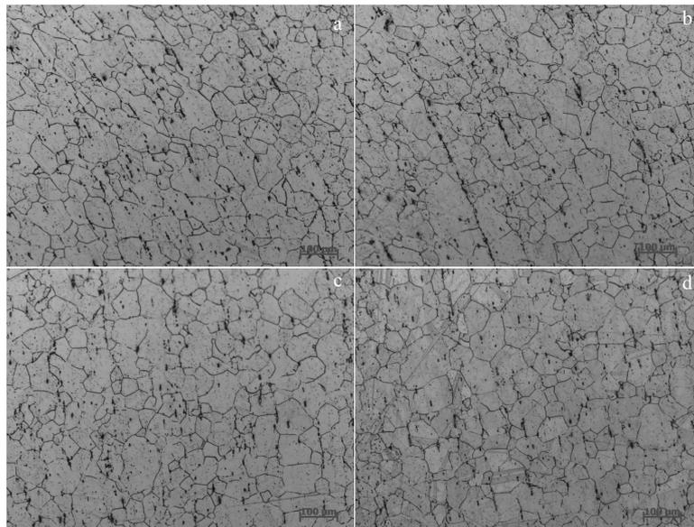
Fig.9 Microstructures of the outer zone of the welded joint: (a) area A, (b) area B, (c) area C, and (d) area D
