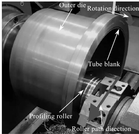
Fig.4 Assembly diagram of serrated groove spinning
