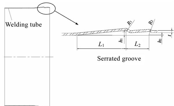
Fig.1 Section profile of the serrated groove
