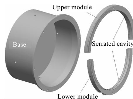
Fig.3 Serrated groove inner spinning dies
