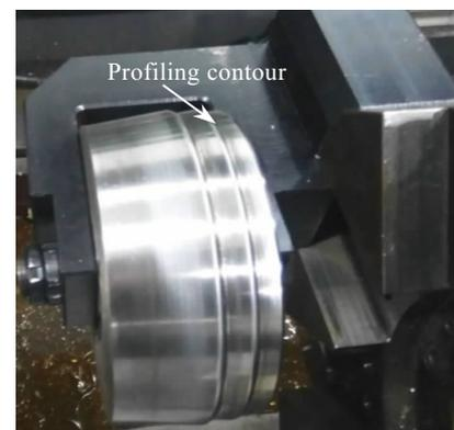
Fig.2 Profiling roller
