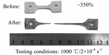
Fig.4 Tensile specimens of Ti-43.5Al-8Nb-0.2W alloy with a grain size of  $\sim 5 \mu\text{m}$  before and after tension at  $1000 \text{ }^\circ\text{C}/2\times 10^{-4} \text{ s}^{-1}$  (note that glass lubricant was applied to protect the surface oxidation during tension)
