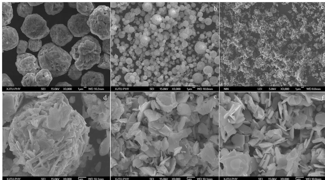
Fig.1 SEM images of original precursor powders (a~c) and precursor powders after heat treatment at 780 °C for 10 h in a flowing 0.1%  $\text{O}_2$ /balance  $\text{N}_2$  atmosphere (d~f): (a, d) powder 1, (b, e) powder 2 and (c, f) powder 3
