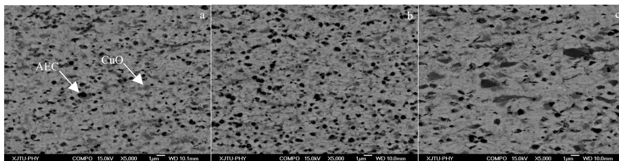
Fig.2 SEM images of bulks pressed by precursor powders after heat treatment: powder 1 (a), powder 2 (b), and powder 3 (c)
