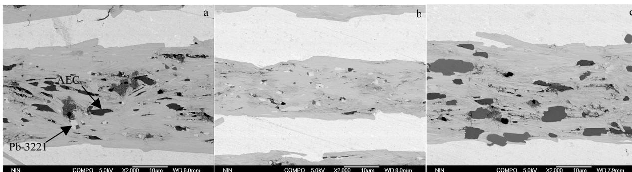
Fig.5 SEM images of three kinds of tapes: (a) tape A from powder 1, (b) tape B from powder 2, and (c) tape C from powder 3
