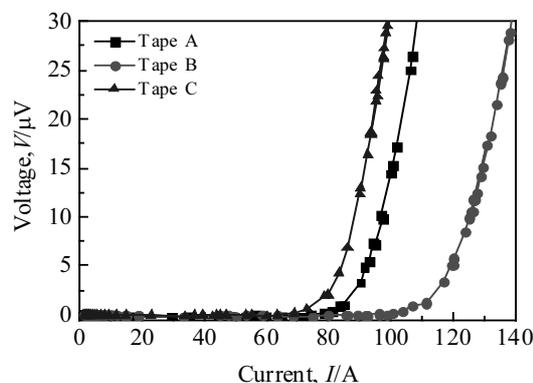
Fig.4 *I-V* curves of 37-filaments tapes (A, B, C), corresponding to powder 1, powder 2 and powder 3
