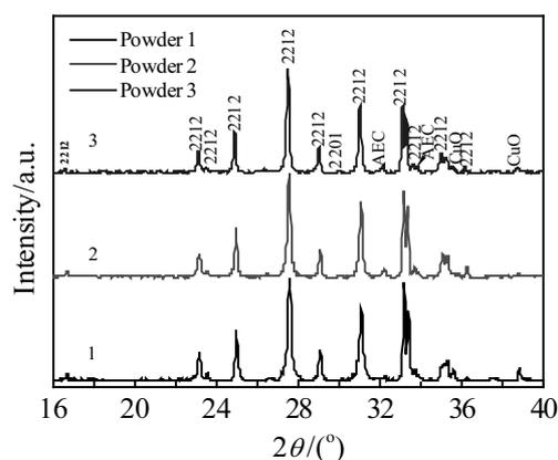
Fig.3 XRD pattern of powder 1, powder 2 and powder 3 after heat treatment at 780 °C for 10 h in a flowing 0.1% O<sub>2</sub>/balance N<sub>2</sub> atmosphere
