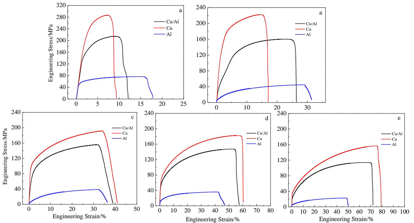
Fig.6 Engineering stress-strain curves of clad sheet and individual components at different annealing temperatures in tension tests: (a) 300 °C, (b) 320 °C, (c) 340 °C, (d) 360 °C, and (e) 400 °C
