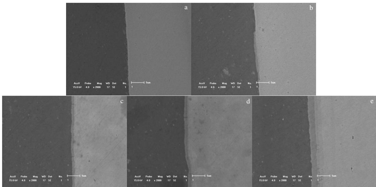
Fig.1 SEM interfacial microstructures of Cu/Al clad sheet annealed at different temperatures: (a) 300 °C, (b) 320 °C, (c) 340 °C, (d) 360 °C, and (e) 400 °C
