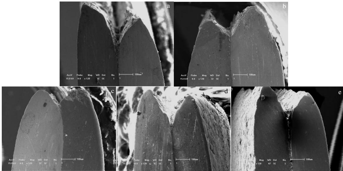
Fig.8 SEM fractographs of clad sheet at different annealing temperatures along tensile axis: (a) 300 °C, (b) 320 °C, (c) 340 °C, (d) 360 °C, and (e) 400 °C
