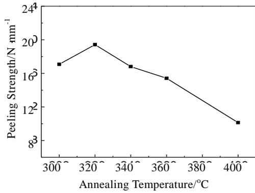
Fig.3 Variation of peeling strength of Cu/Al clad sheets with different annealing temperatures
