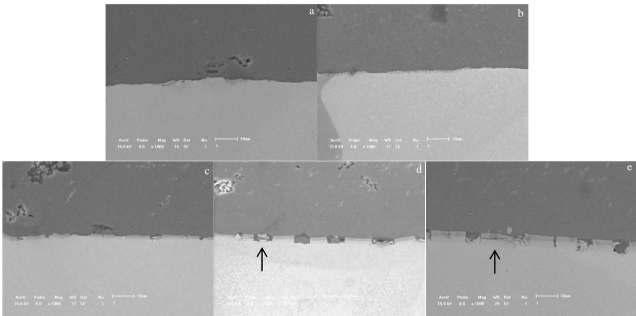
Fig.9 Interfacial microstructures of clad sheet near tensile fracture at different annealing temperatures: (a) 300 °C, (b) 320 °C, (c) 340 °C, (d) 360 °C, and (e) 400 °C
