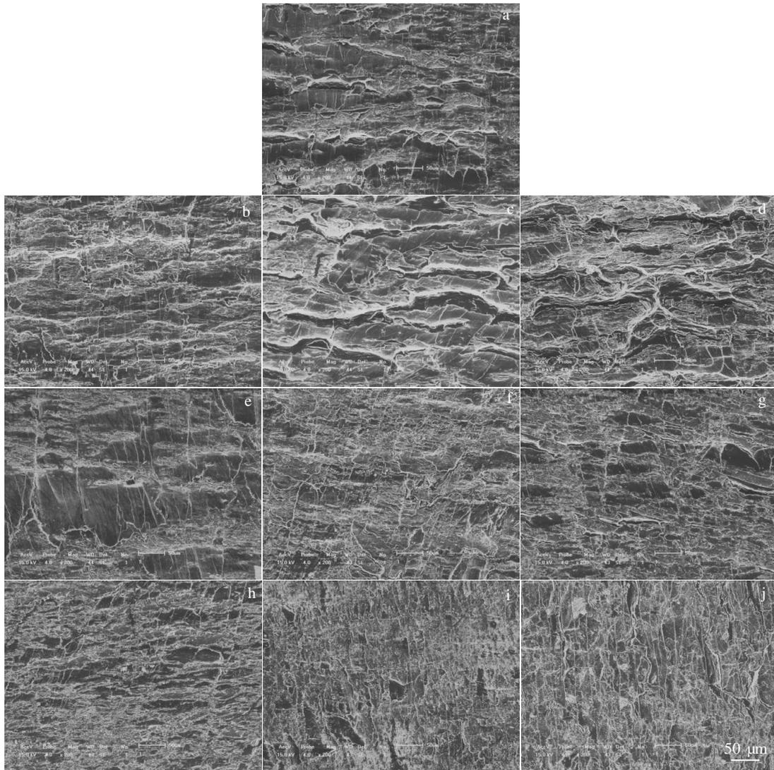
Fig.4 SEM microstructures of peeled surface of Cu/Al clad sheet annealed at different temperatures: (a) 300 °C Cu, (b) 300 °C Al, (c) 320 °C Cu, (d) 320 °C Al, (e) 340 °C Cu, (f) 340 °C Al, (g) 360 °C Cu, (h) 360 °C Al, (i) 400 °C Cu, and (j) 400 °C Al
