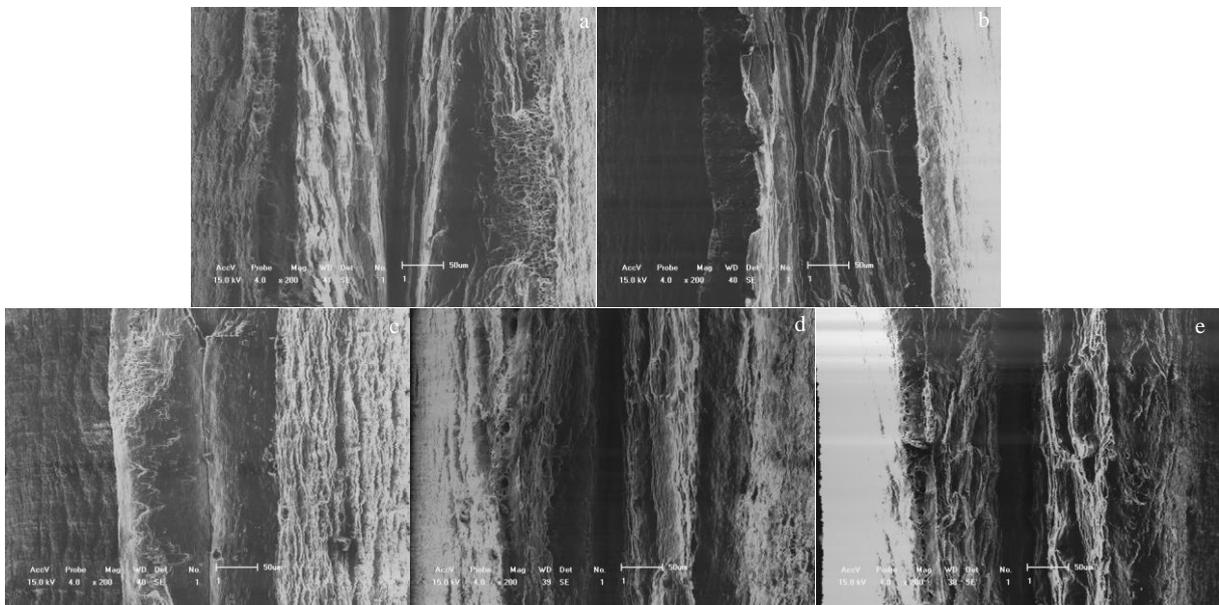
Fig.7 SEM fractographs of clad sheet at different annealing temperatures vertical to tensile axis: (a) 300 °C, (b) 320 °C, (c) 340 °C, (d) 360 °C, and (e) 400 °C
