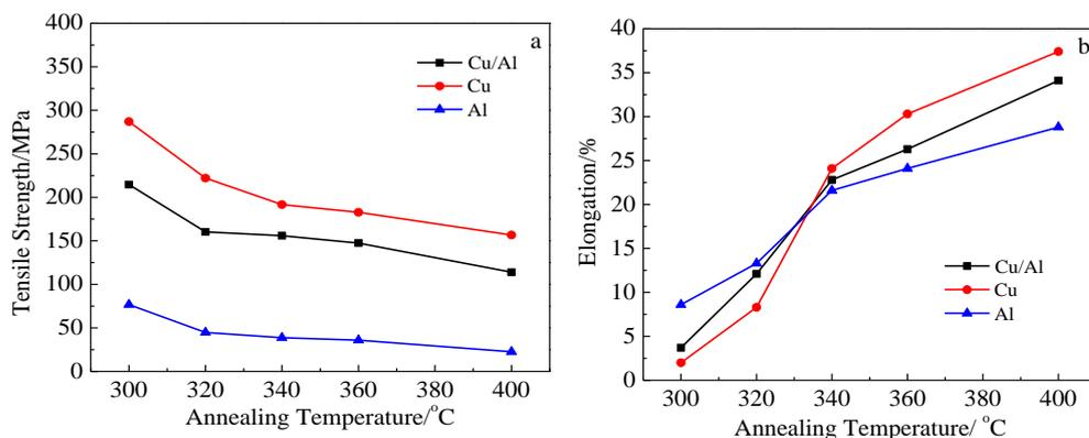
Fig.5 Variation of tensile properties of clad sheet at different annealing temperatures: (a) tensile strength and (b) elongation
