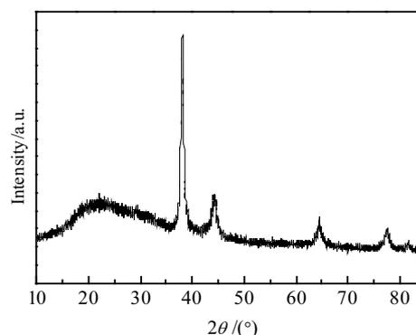
Fig.2 XRD pattern of gold nanoparticles
