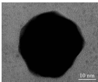
Fig.6 HRTEM image of gold nanoparticles
