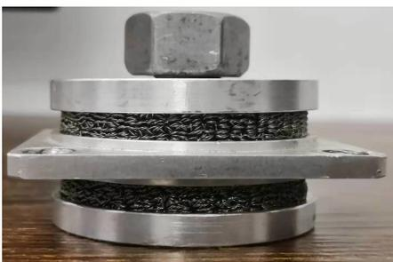
Fig.2 Picture of the SMA-MR damper
