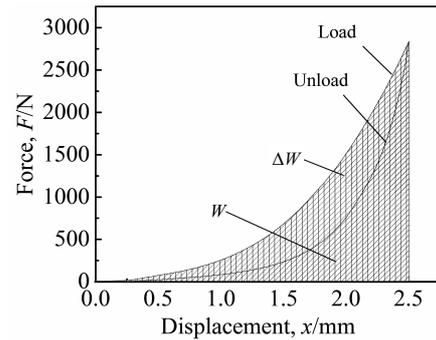
Fig.3 Hysteresis loop of the SMA-MR damping
