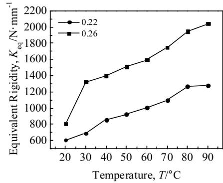
Fig.7 Equivalent rigidity curves of SMA-MR at different temperatures
