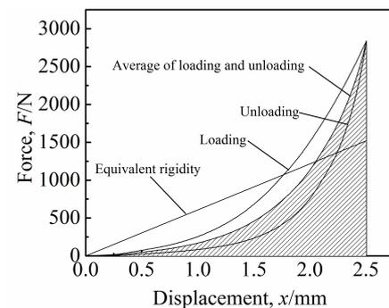
Fig.4 Solution principle of equivalent rigidity curve
