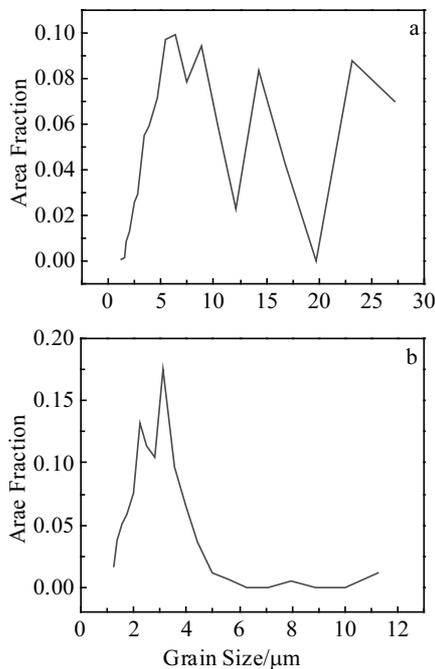
Fig.9 Grain size distribution line charts after 4 passes (a) and 8 passes (b)
