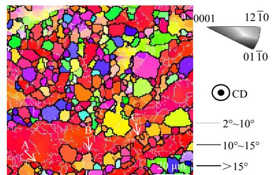
Fig.3 Orientation map of Mg-1Zn-1Gd alloy deformed after extrusion to 4 passes
