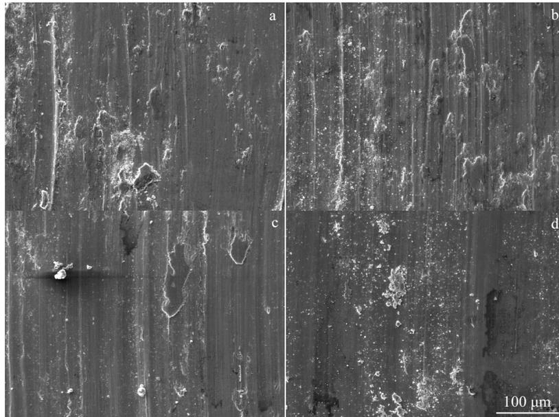
Fig.4 Worn surface of Ti alloys with different RHAs SiO<sub>2</sub> addition: (a) 0 wt%, (b) 0.25 wt%, (c) 0.5 wt%, and (d) 1.0 wt%
