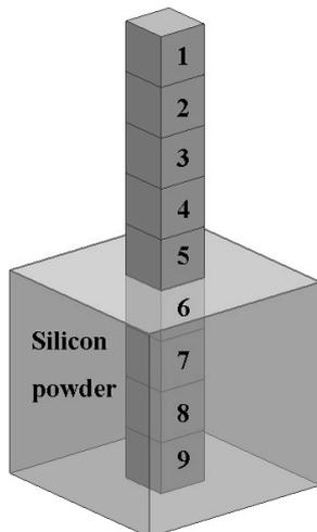
Fig.1 Schematic diagram of the relative position between silicon powder and C/C preform
