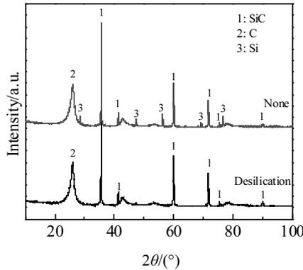
Fig.7 XRD patterns of C/SiC composites before and after desilication
