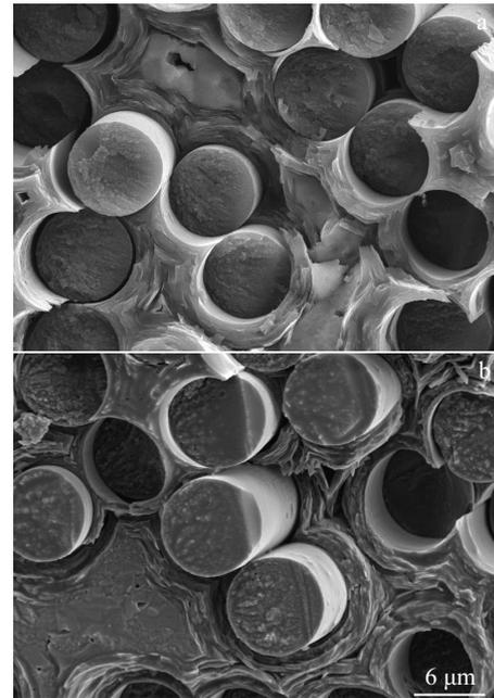
Fig.9 Fracture morphologies of sample after bending test: (a) before desilication and (b) after desilication
