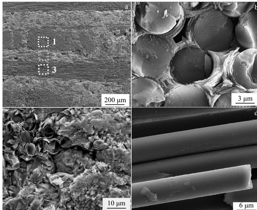
Fig.4 SEM images of surface morphologies of C/SiC composite (a) and enlarged view of the dashed box 1 (b), 2 (c), and 3 (d) in Fig.4a
