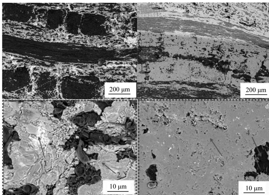
Fig.6 BEM of C/SiC composite material before (a, c) and after (b, d) desilication
