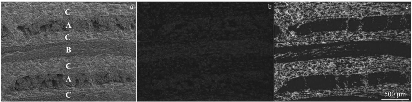
Fig.3 SEM image of C/SiC composite (a) and its element mapping of C (b) and Si (c)
