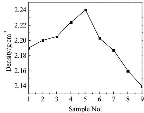
Fig.2 Density change of C/SiC composite along the embedding position in silicon powder
