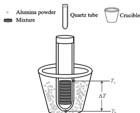
Fig.1 Schematic diagram of the temperature difference ( $\Delta T$ ) between surface temperature ( $T_s$ ) and bottom temperature ( $T_b$ ) of the mixture
