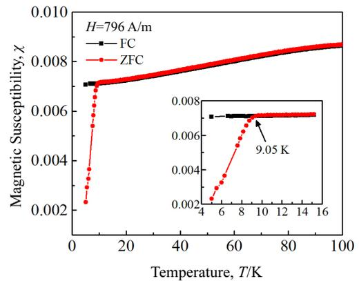
Fig.9 Magnetic susceptibility-temperature curve of FeSe crystals with zero-field-cooling (ZFC) and field-cooling (FC)
