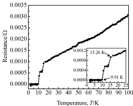
Fig.8 Resistance-temperature curve of FeSe crystals
