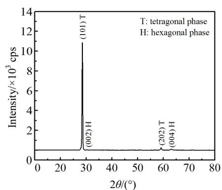
Fig.5 XRD pattern of the cleavage plane of FeSe crystal
