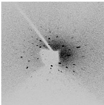
Fig.7 Laue diffraction pattern of a thin FeSe single crystal
