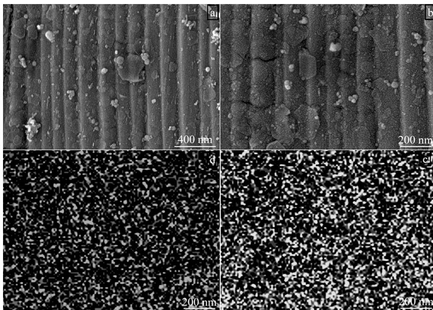
Fig.3 SEM images of FeSe crystals (a, b) and EDS mapping of Fe (c) and Se (d) in Fig.3b
