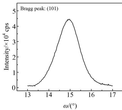
Fig.6 XRD rocking curve of the (101) reflection for the FeSe crystal
