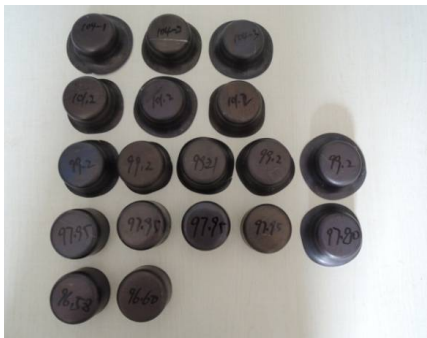
Fig.11 Drawing test piece of Ti-Al clad plate
