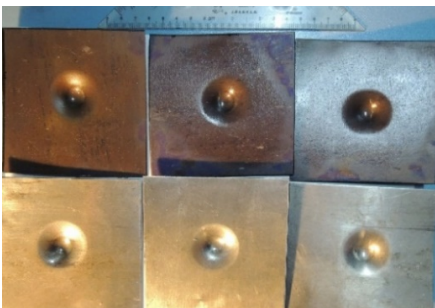
Fig.10 Cupping test piece of Ti-Al clad plate
