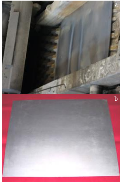
Fig.5 Hot rolled Ti-Al clad plate: (a) hot rolled plate, (b) plate after levelling
