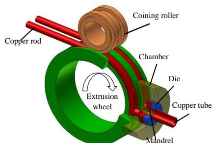
Fig.1 Principle of copper tube continuous extrusion using double billets
