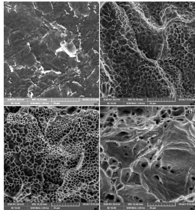
Fig.7 Fracture morphologies of the weld seam at different positions: (a) position A, (b) position B, (c) position C, and (d) position D
