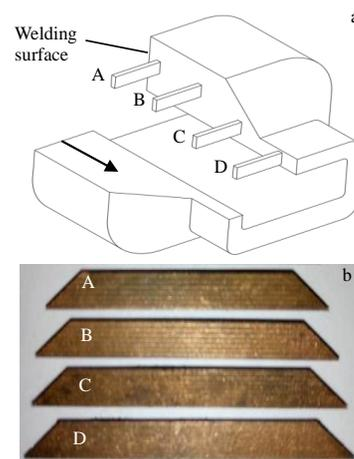
Fig.3 Sampling diagram (a) and specimens at different locations (b)
