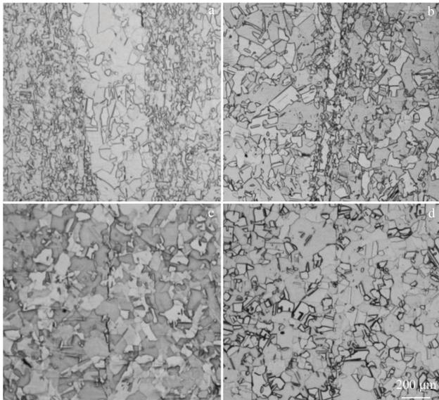
Fig.4 Microstructure evolution of weld seam in continuously extruded copper tube at different positions marked in Fig.3a: (a) position A, (b) position B, (c) position C, and (d) position D
