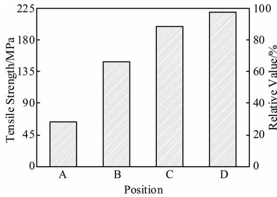
Fig.6 Tensile strength of weld seam at different positions
