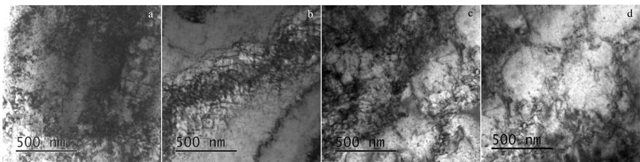
Fig.5 TEM microstructures of weld zone at different positions marked in Fig.3a: (a) position A, (b) position B, (c) position C, and (d) position D
