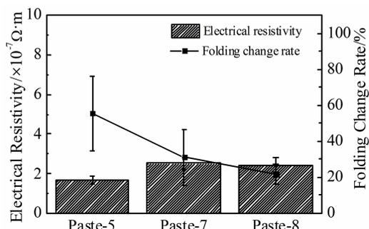
Fig.13 Electrical resistivity and folding change rate of Paste-5, Paste-7, and Paste-8 specimens
