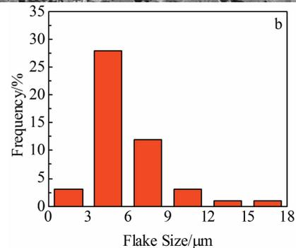
Fig.7 Surface morphology (a) and flake size distribution (b) of Paste-5 specimen
