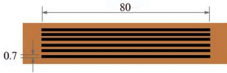
Fig.1 Schematic diagram of silver paste lines on PI substrate
