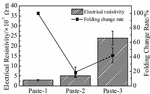
Fig.5 Electrical resistivity and folding change rate of Paste-1, Paste-2, and Paste-3 specimens
