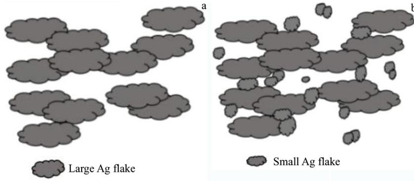
Fig.8 Schematic diagrams of before (a) and after (b) adding small Ag flakes for improvement in electrical conductivity of silver paste
