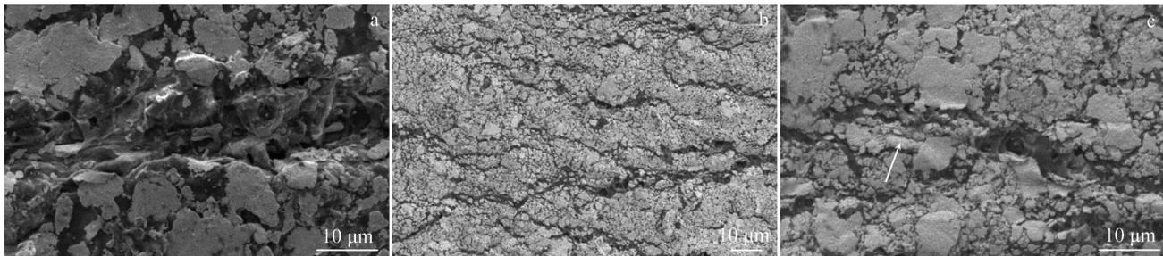
Fig.10 SEM surface morphologies of different silver pastes after folding: (a) Paste-1, (b) Paste-2, and (c) Paste-5
