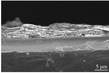
Fig.4 Cross-section morphology of Paste-1 specimen
