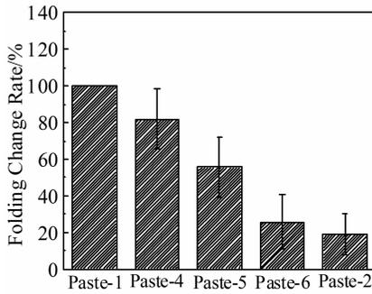
Fig.9 Folding change rate of mixed silver pastes with Ag flakes of 10 and 5 μm in length
