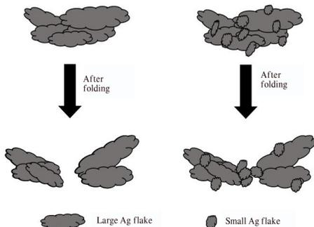
Fig.11 Schematic diagram of adding small Ag flakes for improvement in electrical conductivity of silver paste after folding
