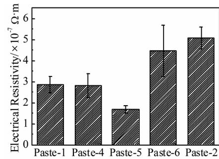
Fig.6 Electrical resistivity of mixed silver pastes with Ag flakes of 10 and 5  $\mu m$  in length
