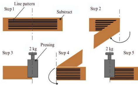
Fig.2 Schematic diagram of folding process
