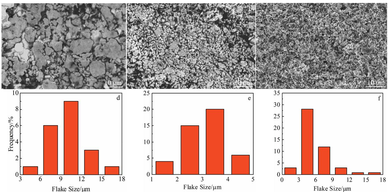
Fig.3 Surface morphologies (a-c) and flake size distributions (d-f) of Paste-1 (a, d), Paste-2 (b, e), and Paste-3 (c, f) specimens
