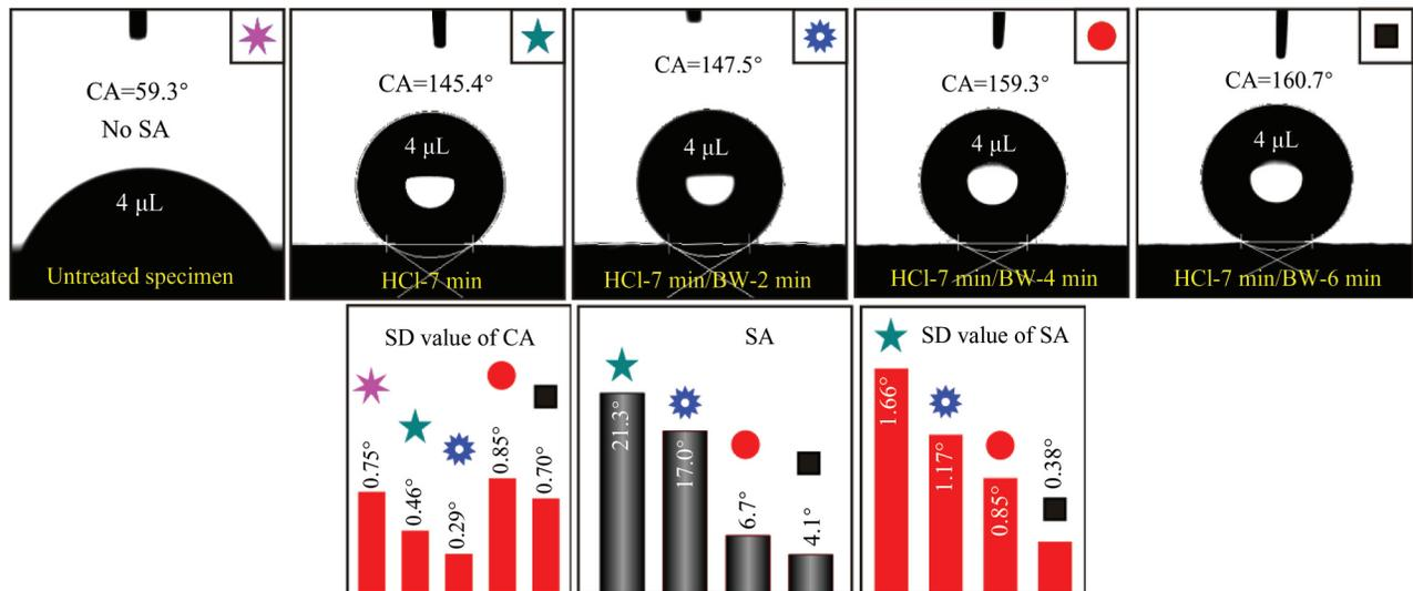
Fig.3 Wettability of 7075 Al alloys after different etching processes and comparison results of SA, SD value of CA, and SD value of SA (BW: boiling water)
