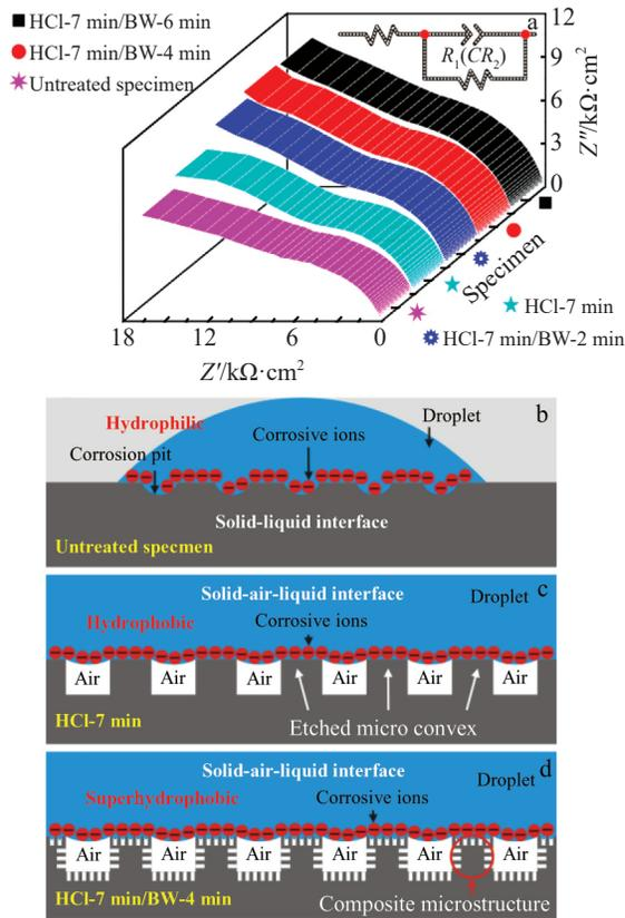
Fig.4 Impedance spectra of 7075 Al alloys after different etching processes (a); anticorrosion mechanisms of untreated specimen (b), hydrophobic alloy (c), and superhydrophobic alloy (d)
