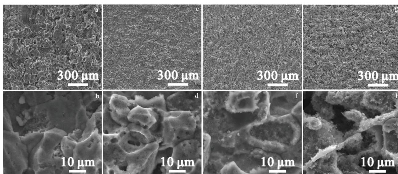
Fig.1 SEM images of 7075 Al alloys after different treatments: (a, b) HCl-7 min, (c, d) HCl-7 min/boiling water-2 min, (e, f) HCl-7 min/boiling water-4 min, and (g, h) HCl-7 min/boiling water-6 min
