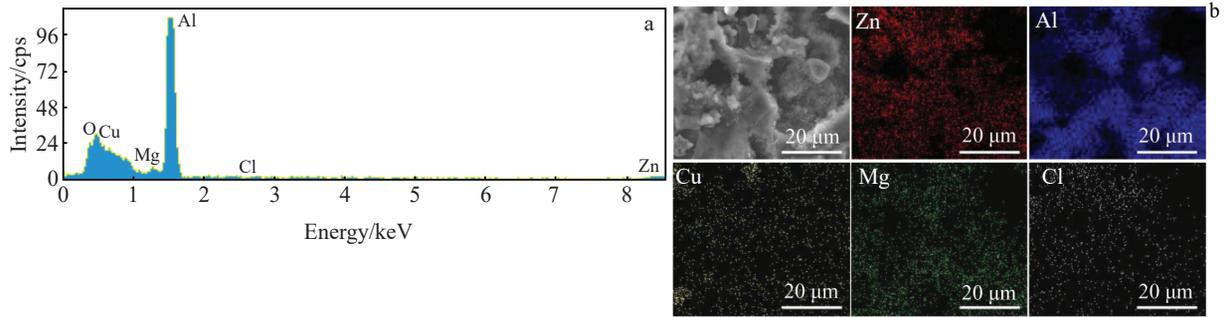
Fig.2 EDS spectrum (a) and element distributions (b) of 7075 Al alloy after immersion treatment of HCl-7 min/boiling water-4 min
