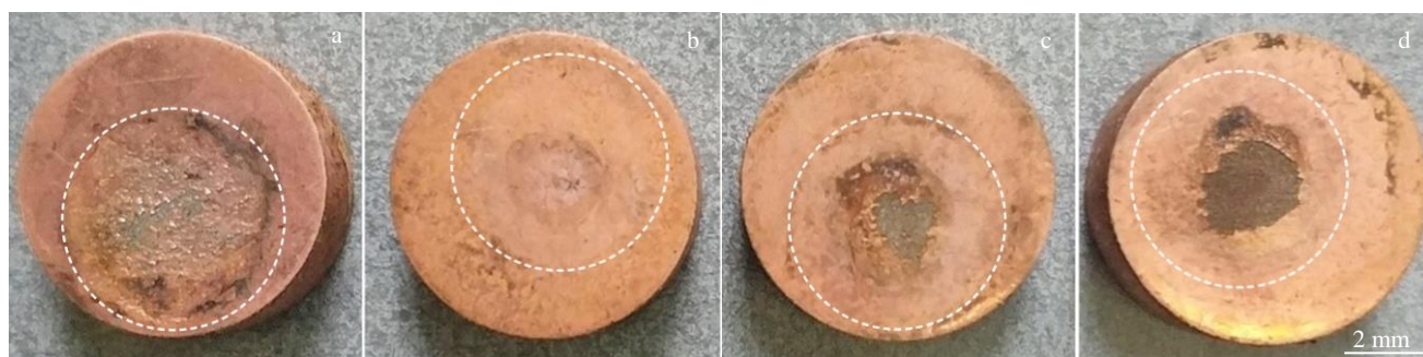
Fig.11 Macroscopic corrosion morphologies of sintered NdFeB protected by Cu-GR composites with different graphene concentrations: (a) 0 \text{ g}\cdot\text{L}^{-1} , (b) 0.3 \text{ g}\cdot\text{L}^{-1} , (c) 0.6 \text{ g}\cdot\text{L}^{-1} , and (d) 0.9 \text{ g}\cdot\text{L}^{-1}
