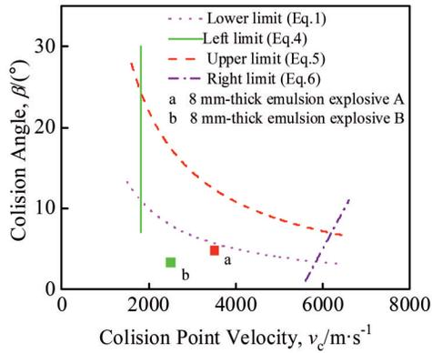
Fig.3 T2/Q345 explosive welding window
