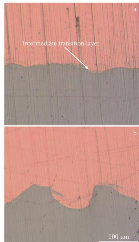
Fig.4 Microstructures of the interface of T2/Q345 clad plate: (a) close to initiation end and (b) away from initiation end
