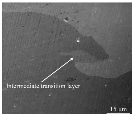
Fig. 5 SEM image of the interface of T2/Q345 clad plate
