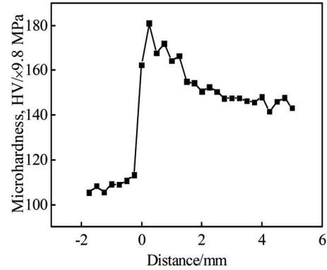
Fig.10 Microhardness of T2/Q345 explosive welding interface
