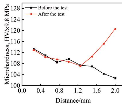
Fig.11 Microhardness changes of tensile shear specimens
