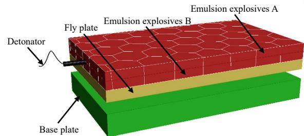
Fig.2 Schematic diagram of explosive welding set-up with double-layer honeycomb emulsion explosive
