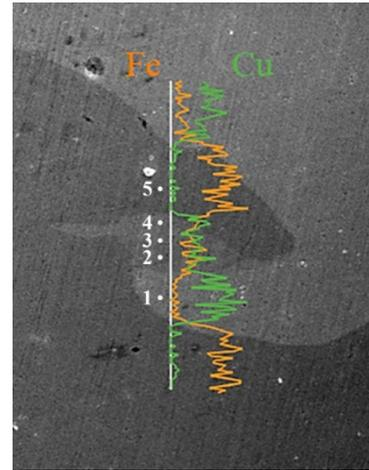
Fig. 6 EDS line scanning across the interface of T2/Q345 clad plate
