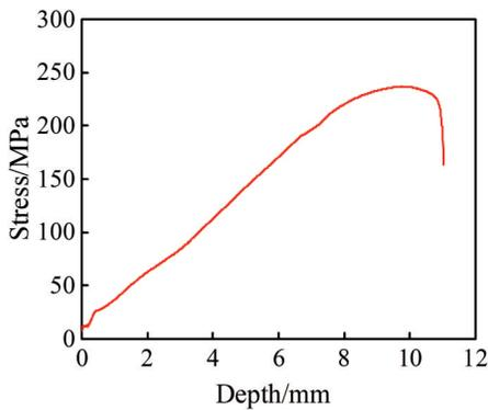
Fig.8 Stress-displacement curve of tensile shear specimen
