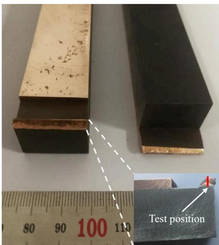
Fig.9 Physical diagram of tensile shear failure specimen
