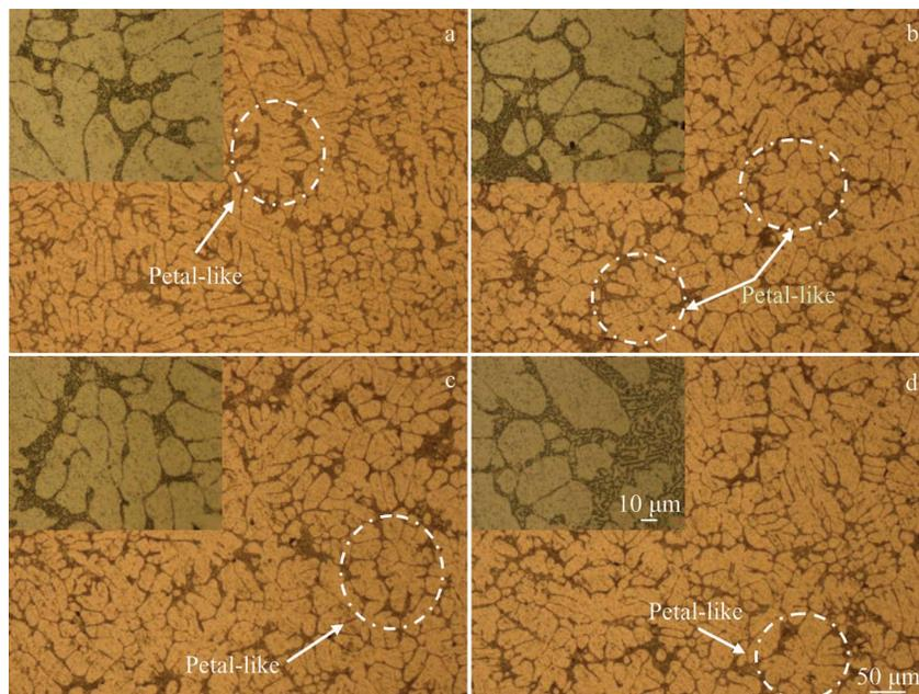
Fig.2 As-cast microstructure of A356-0.3Yb alloy with different contents of Zr: (a) 0.15wt%, (b) 0.25wt%, (c) 0.35wt%, and (d) 0.45wt%
