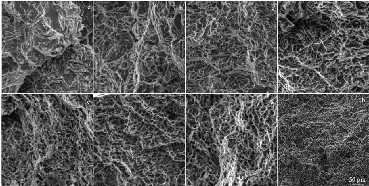
Fig.7 Tensile fracture morphologies of alloys with different refinement and modification treatments (T6): (a) A356, (b) A356-0.1Yb, (c) A356-0.3Yb, (d) A356-0.5Yb, (e) A356-0.3Yb-0.15Zr, (f) A356-0.3Yb-0.25Zr, (g) A356-0.3Yb-0.35Zr, and (h) A356-0.3Yb-0.45Zr
