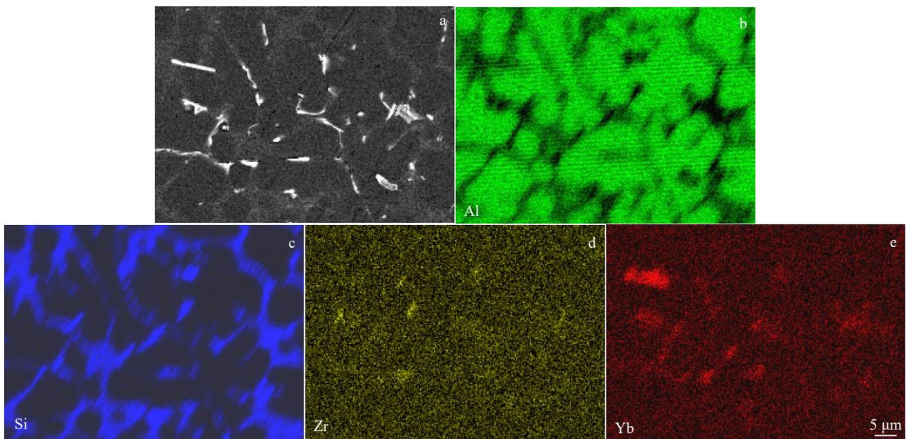
Fig.8 SEM image (a) and EDS element mappings of Al (b), Si (c), Zr (d) and Yb (e) for A356-0.3Yb-0.25Zr
