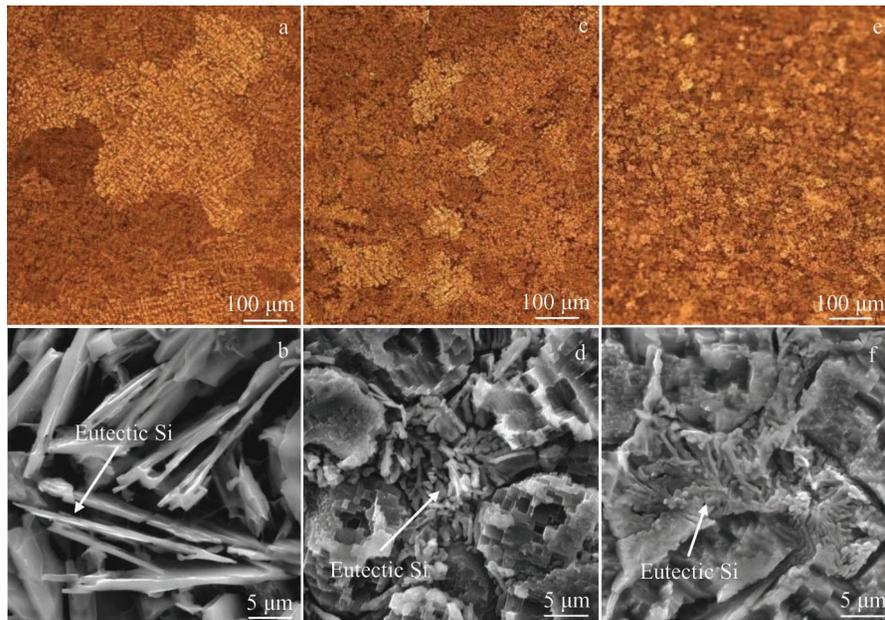
Fig.3 Microstructures of alloys after deep corrosion: (a, b) A356, (c, d) A356-0.3Yb, and (e, f) A356-0.3Yb-0.25Zr
