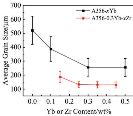
Fig.4 Effect of Yb and Zr content on average grain size of alloy
