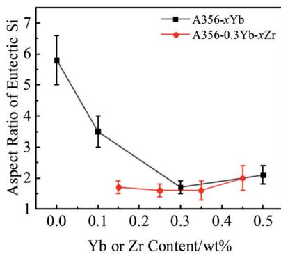
Fig.5 Influence of Yb and Zr content on aspect ratio of eutectic Si
