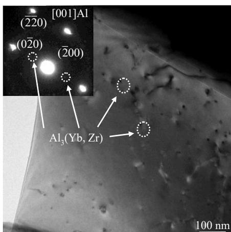
Fig.10 TEM image of precipitates in A356-0.3Yb-0.25Zr alloy after heat treatment (T6)
