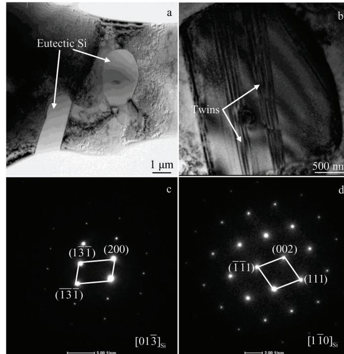
Fig.9 Bright-field TEM images of silicon phase taken in A356 (a) and A356-0.3Yb-0.25Zr (b) alloys; SAED patterns of eutectic silicon in A356-0.3Yb-0.25Zr alloys along  $[01\bar{3}]_{\text{Si}}$  (c) and  $[1\bar{1}0]_{\text{Si}}$  (d)
