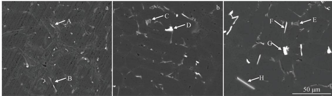
Fig.6 SEM images of alloys with different refinement and modification treatments: (a) A356, (b) A356-0.3Yb, and (c) A356-0.3Yb-0.25Zr
