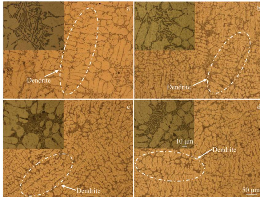
Fig.1 As-cast microstructures of A356 alloy with different contents of Yb: (a) 0.0wt%, (b) 0.1wt%, (c) 0.3wt%, and (d) 0.5wt%
