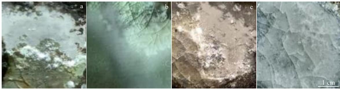
Fig.7 Surface morphologies of 304 stainless steel plate after reacting with different flux: (a) flux No.1 at 700 °C, (b) flux No.2 at 700 °C, (c) flux No.3 at 700 °C, and (d) flux No.3 at 540 °C
