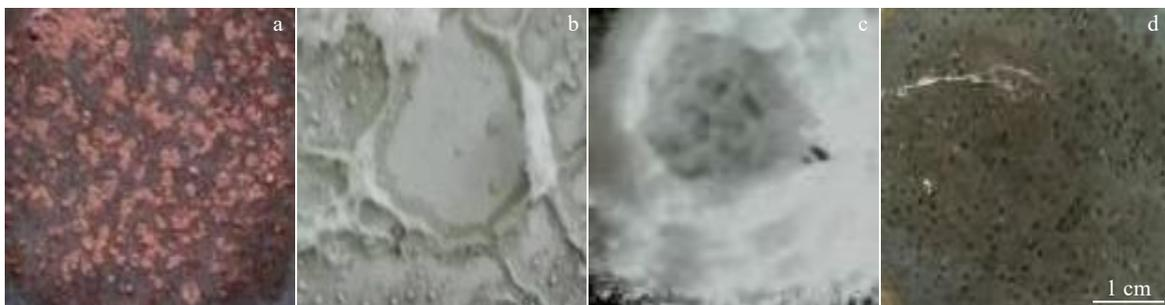
Fig.3 Surface morphologies of 304 stainless steel plate reacted with different fluxes at 700 °C: (a) KF, (b)  $\text{KHF}_2$ , (c)  $\text{K}_2\text{B}_4\text{O}_7$ , and (d)  $\text{H}_3\text{BO}_3$
