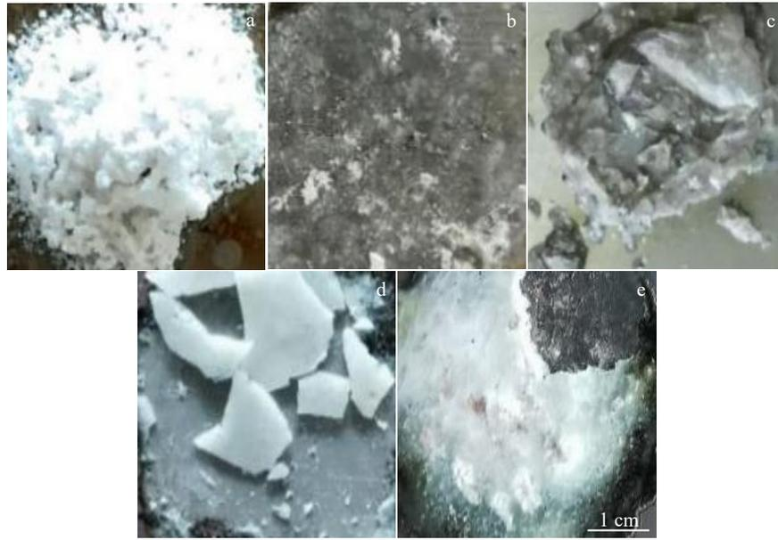
Fig.5 Surface morphologies of 304 stainless steel plate after reaction with different fluxes: (a)  $K_2B_4O_7:H_3BO_3=10:7$ , (b)  $H_3BO_3:KF=7:3$ , (c)  $H_3BO_3:KHF_2=7:3$ , (d)  $K_2B_4O_7:KHF_2=10:3$ , and (e)  $K_2B_4O_7:KF=10:3$
