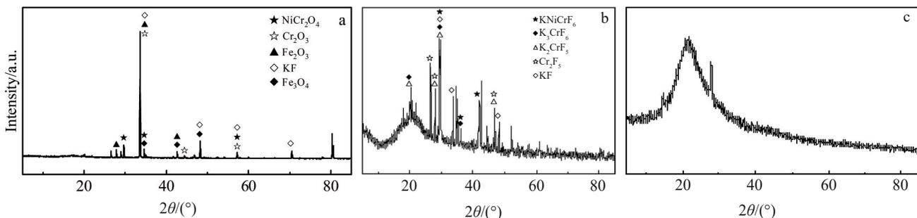
Fig.4 XRD patterns of reaction product between flux and oxide film at 700 °C: (a) KF, (b)  $\text{KHF}_2$ , and (c)  $\text{H}_3\text{BO}_3$
