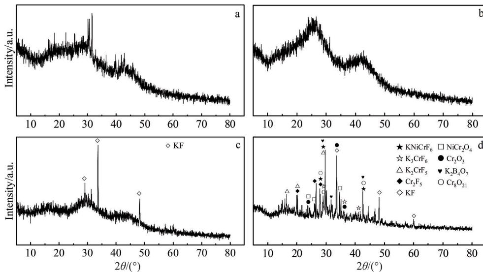
Fig.6 XRD patterns of reaction product between flux and oxide film: (a)  $H_3BO_3:KF=7:3$ , (b)  $H_3BO_3:KHF_2=7:3$ , (c)  $K_2B_4O_7:KHF_2=10:3$ , and (d)  $K_2B_4O_7:KF=10:3$
