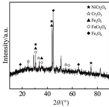
Fig. 2 XRD pattern of oxide film on 304 stainless steel surface heated at 700 °C
