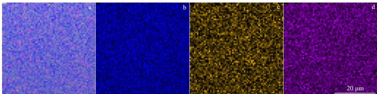
Fig.1 EDS results of element distribution of 304 stainless steel heated at 700 °C: (a) total element, (b) Fe, (c) Ni, and (d) Cr
