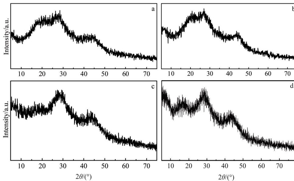
Fig.8 XRD patterns of reaction product between flux and oxide film: (a) flux No.1 at 700 °C, (b) flux No.2 at 700 °C, (c) flux No.3 at 700 °C, and (d) flux No.3 at 540 °C
