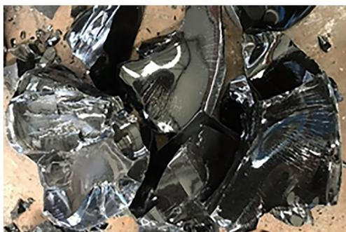
Fig.8 Macroscopic feature of glass slag
