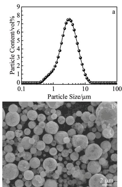
Fig.1 Particle size distribution (a) and morphology (b) of precursor powder prepared by ultrasonic spray pyrolysis
