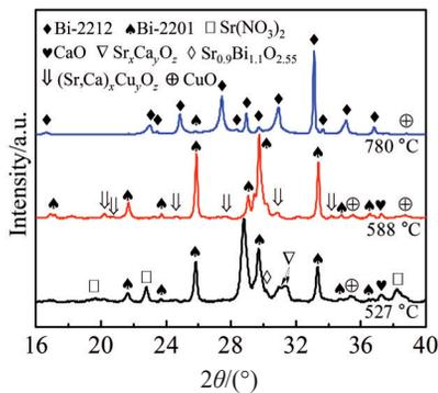
Fig.4 XRD patterns of precursor powders after heat treatments at 527, 588, and 780 °C for 12 h
