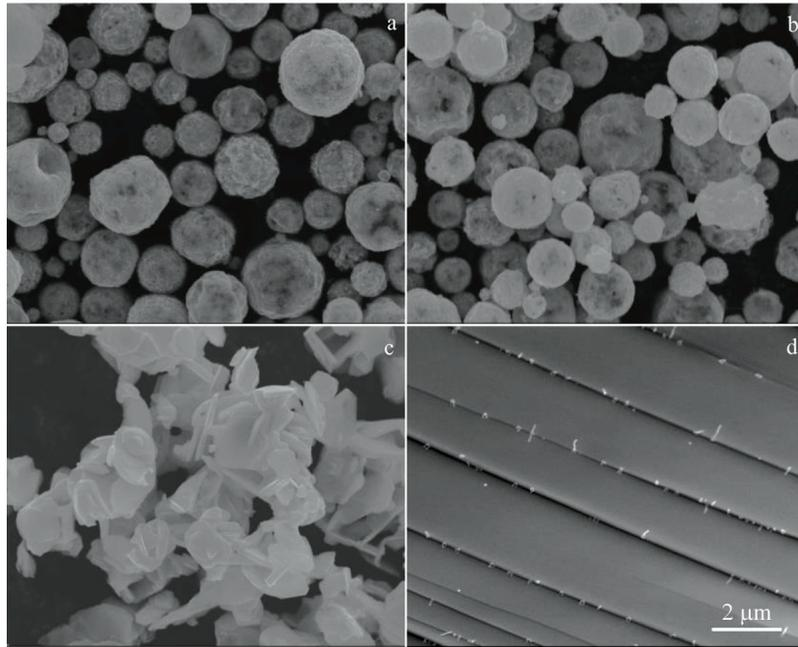
Fig.3 SEM morphologies of precursor powders after heat treatment at different temperatures for 12 h: (a) 527 °C, (b) 588 °C, (c) 780 °C, and (d) 834 °C
