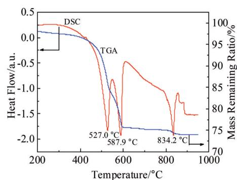
Fig.2 TGA and DSC curves of precursor powders in  $\text{N}_2$ -0.1vol%  $\text{O}_2$  atmosphere at the heating rate of 10 °C/min
