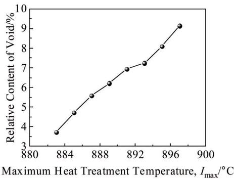
Fig.6 Relationship between relative content of void and  $T_{max}$  of Bi-2212/Ag wire
