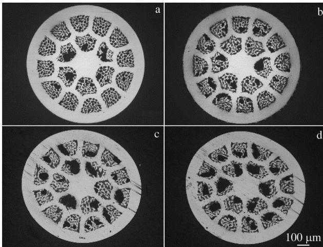
Fig.7 OM images of Bi-2212/Ag wires after heat treatments at different  $T_{max}$ : (a) 883 °C, (b) 887 °C, (c) 891 °C, and (d) 895 °C
