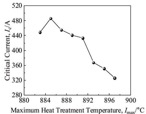
Fig.5 Relationship between  $I_c$  (4.2 K, 0 T) and  $T_{max}$  of Bi-2212/Ag wire
