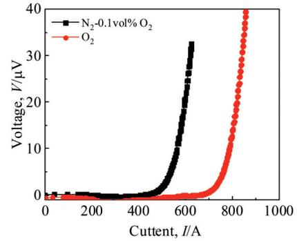
Fig.8  $V$ - $I$  curves of Bi-2212/Ag wires prepared by precursor powders after heat treatment at 770 °C for 12 h in  $N_2$ -0.1vol%  $O_2$  atmosphere and at 860 °C for 12 h in  $O_2$  atmosphere
