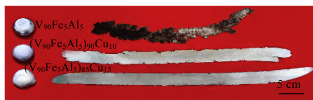
图6 (V_{90}Fe_5Al_5)_{100-x}Cu_x ( x=0, 10, 15 ) 合金铸锭的轧制箔 Fig.6 Rolled foils of (V_{90}Fe_5Al_5)_{100-x}Cu_x ( x=0, 10, 15 ) as-cast ingots [10]
