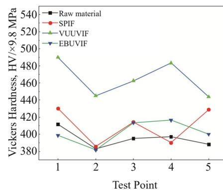
Fig.5 Microhardness results of 6061 aluminum alloy raw material and 6061 aluminum alloys after SPIF, VUUVIF, and EBUVIF processes
