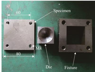
Fig.4 Appearance of specimen and auxiliary tool
