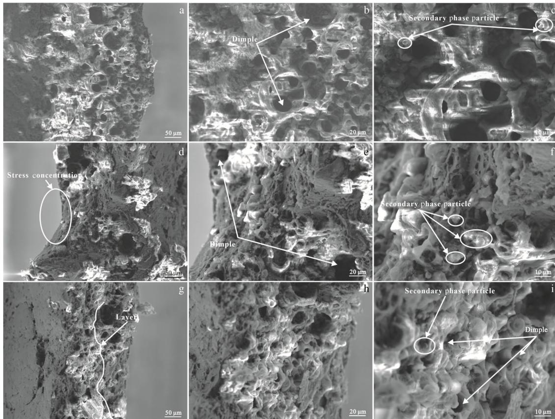
Fig.7 SEM fracture morphologies of 6061 aluminum alloys after SPIF process (a–c), VUUVIF process (d–f), and EBUVIF process (g–i)
