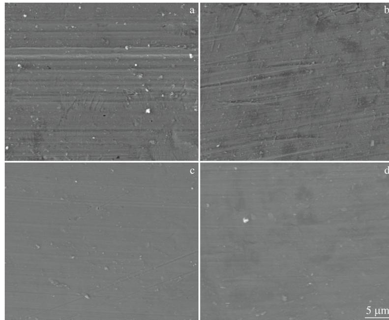
Fig.6 SEM surface morphologies of 6061 aluminum alloy raw material (a) and 6061 aluminum alloys after SPIF (b), VUUVIF (c), and EBUVIF (d) processes
