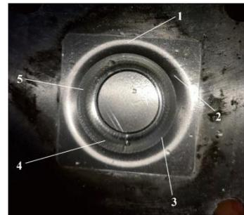
Fig.8 Appearance of specimen and test point positions for residual stress tests
