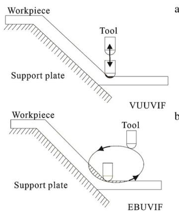
Fig.2 Schematic diagrams of VUUVIF process (a) and EBUVIF process (b)
