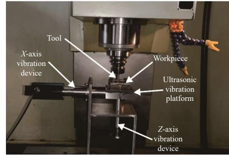
Fig.3 Appearance of ellipse bidirectional ultrasonic vibration system
