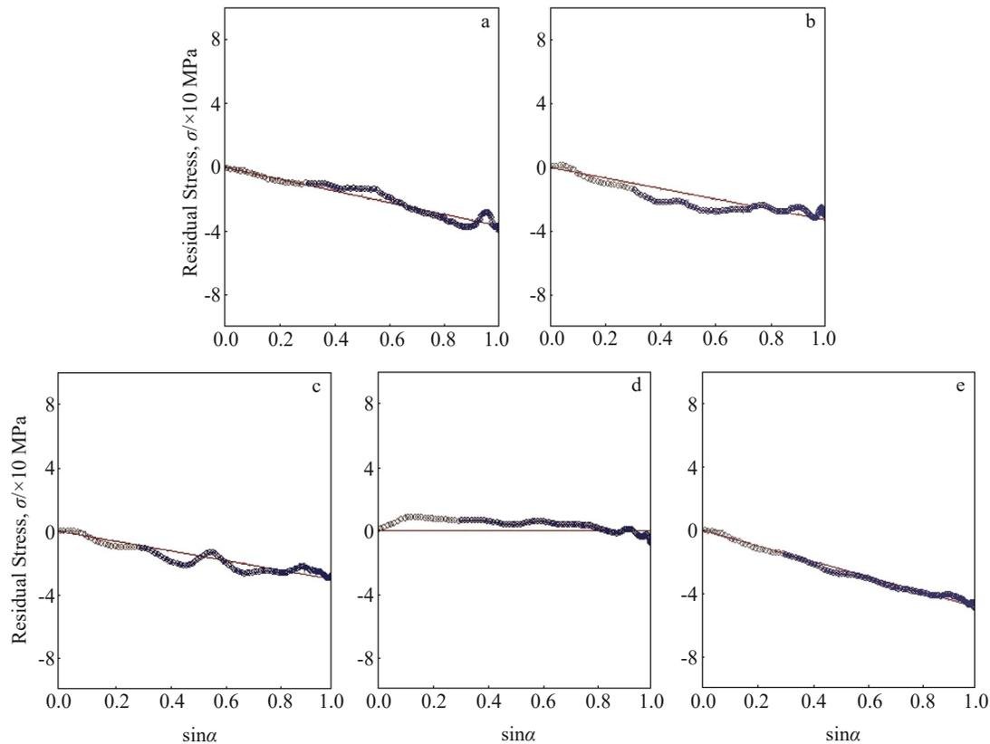
Fig.11 Residual stress curves of point 1 (a), point 2 (b), point 3 (c), point 4 (d), and point 5 (e) of 6061 aluminum alloys after EBUVIF process
