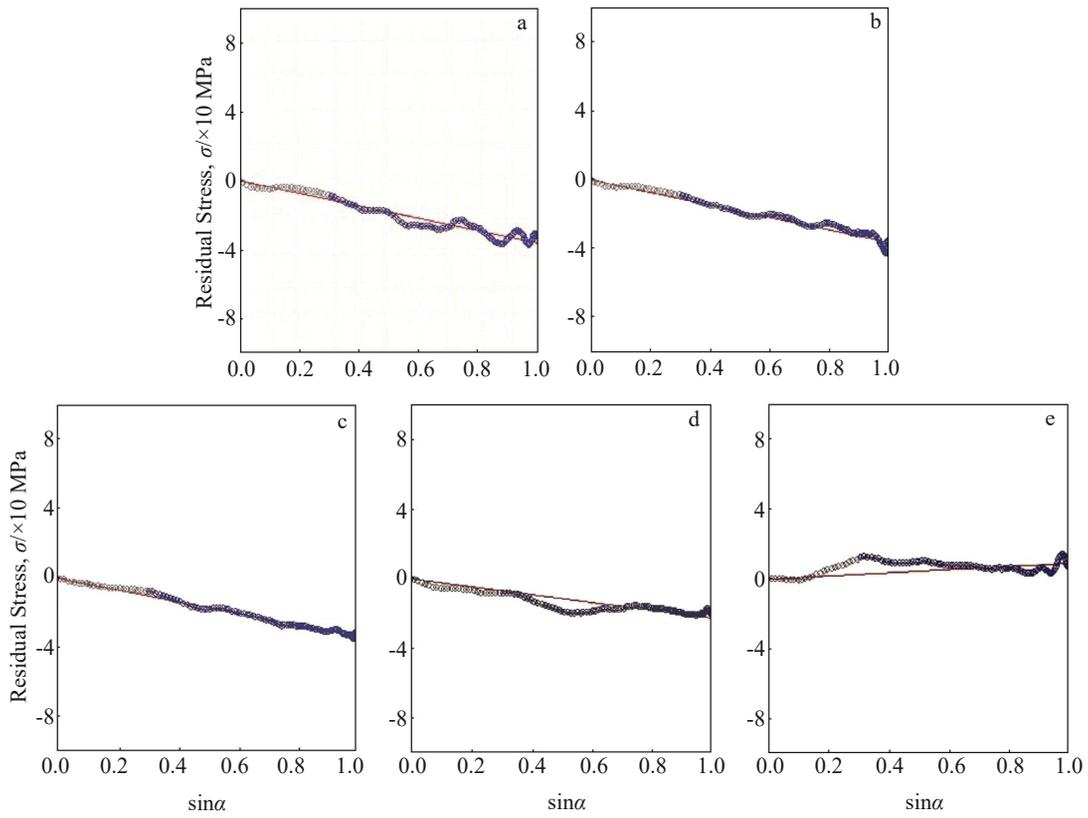
Fig.9 Residual stress curves of point 1 (a), point 2 (b), point 3 (c), point 4 (d), and point 5 (e) of 6061 aluminum alloys after SPIF process
