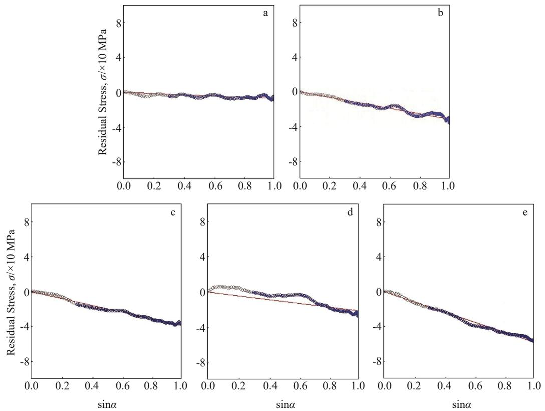
Fig.10 Residual stress curves of point 1 (a), point 2 (b), point 3 (c), point 4 (d), and point 5 (e) of 6061 aluminum alloys after VUUVIF process
