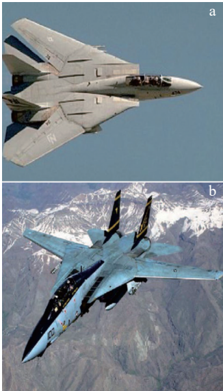
图7 F-14飞机变后掠前后对比 Fig.7 Comparisons of F-14 aircraft before (a) and after (b) changing to sweep [58]
