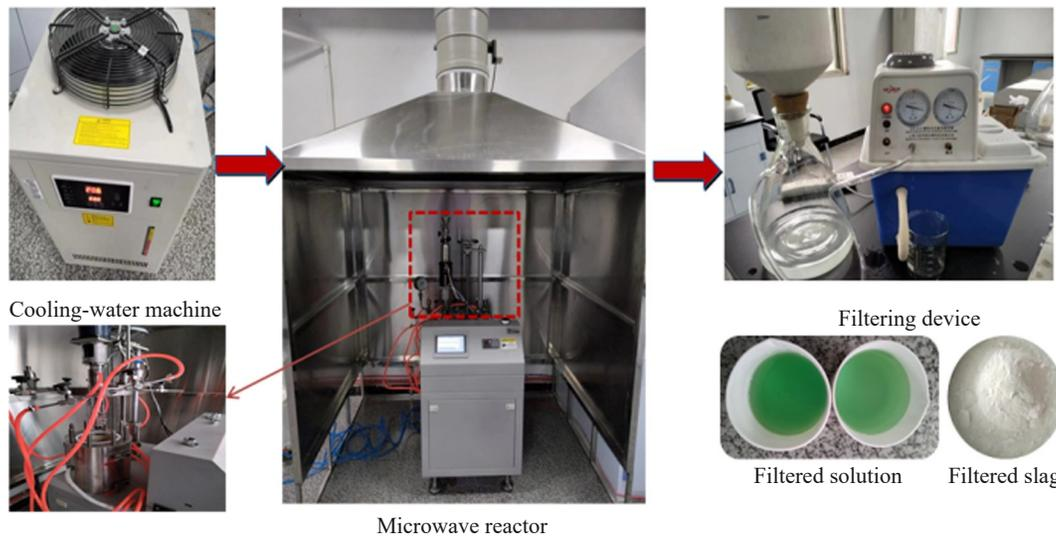
Fig.10 Experimental platform for the microwave reaction for the dissociation of beryllium ore by hydrofluoric acid
