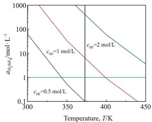
Fig.5 Diagram of metallurgy conditions required for formation of fluorosilicic acid
