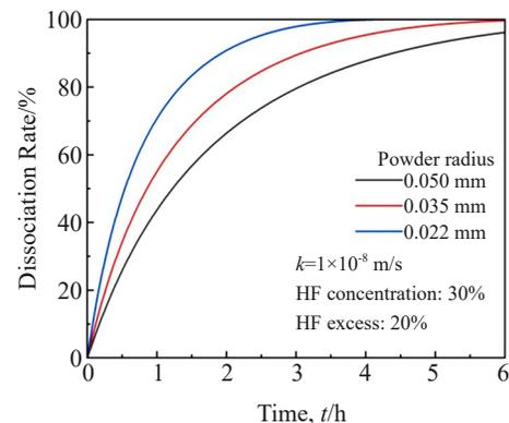
Fig.6 Effect of particle size of ore powder on dissociation rate
