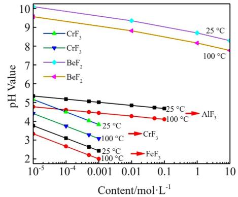
Fig.7 pH range for conversion of different fluorides to hydroxide precipitates
