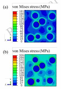
Fig.6 The contour plots of the von Mises stress on the cross section in the *x* direction of the RVE (a) before loading and (b) after loading
