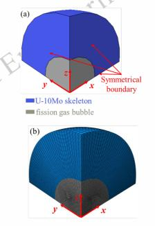
Fig.2 Diagrams of (a) the FE model containing the equivalent solid of fission gas bubble and the U-10Mo skeleton (b) the mesh grid
