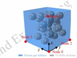
Fig.5 The RVE of irradiated U-10Mo fuels with randomly distributed FGBs According to the homogenization theory, the macroscopic Young's modu-
