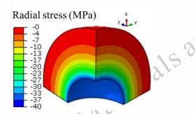
Fig.11 The contour plots of radial stress of the surrounding fuel skeleton before the application of external pressure
