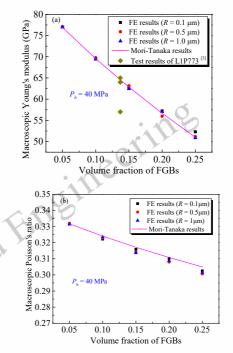
Fig.10 The macroscopic elastic constants of irradiated U-10Mo fuels with different sizes and volume fractions of FGBs (a) macroscopic Young's modulus and (b) macroscopic Poisson's ratio
